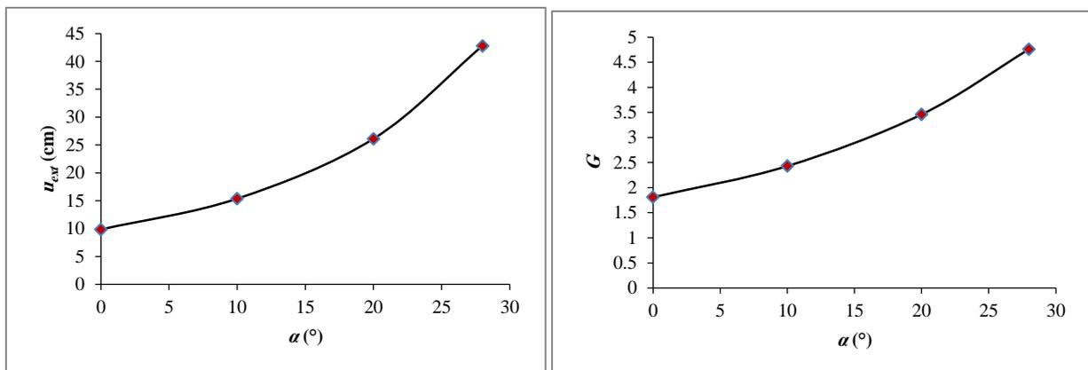
Figure 10. Sensitivity analysis of effect of coal seam dip on main gate roadway stability at  $W=15$  m and  $q=60$  kPa.
