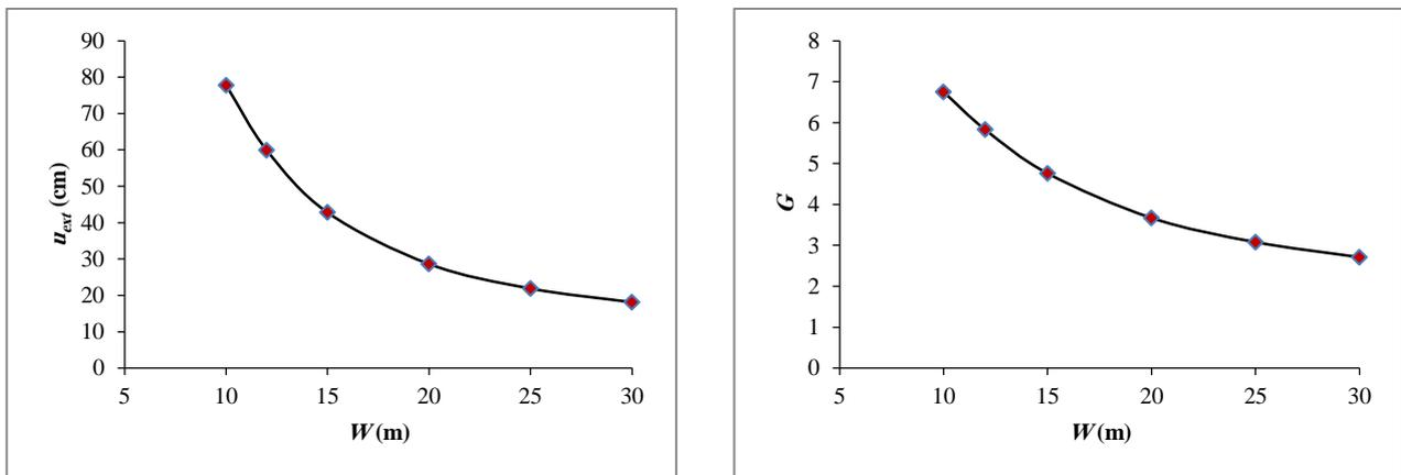
**Figure 7. Sensitivity analysis of pillar width effect on the main gate roadway stability at  $q=60$  kPa.**
