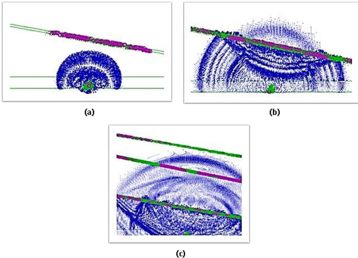
**Figure 4. Wave propagation: a). 0.811 ms after blasting, b). 2.47 ms after blasting and c). 5.11 ms after blasting.**
