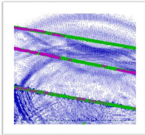
Figure 6. Wave reflection and refraction 6.87 ms after blasting.
