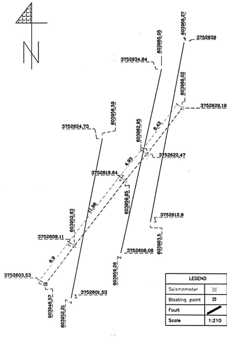
Figure 2. Blasting and geophone locations relating to faults.
