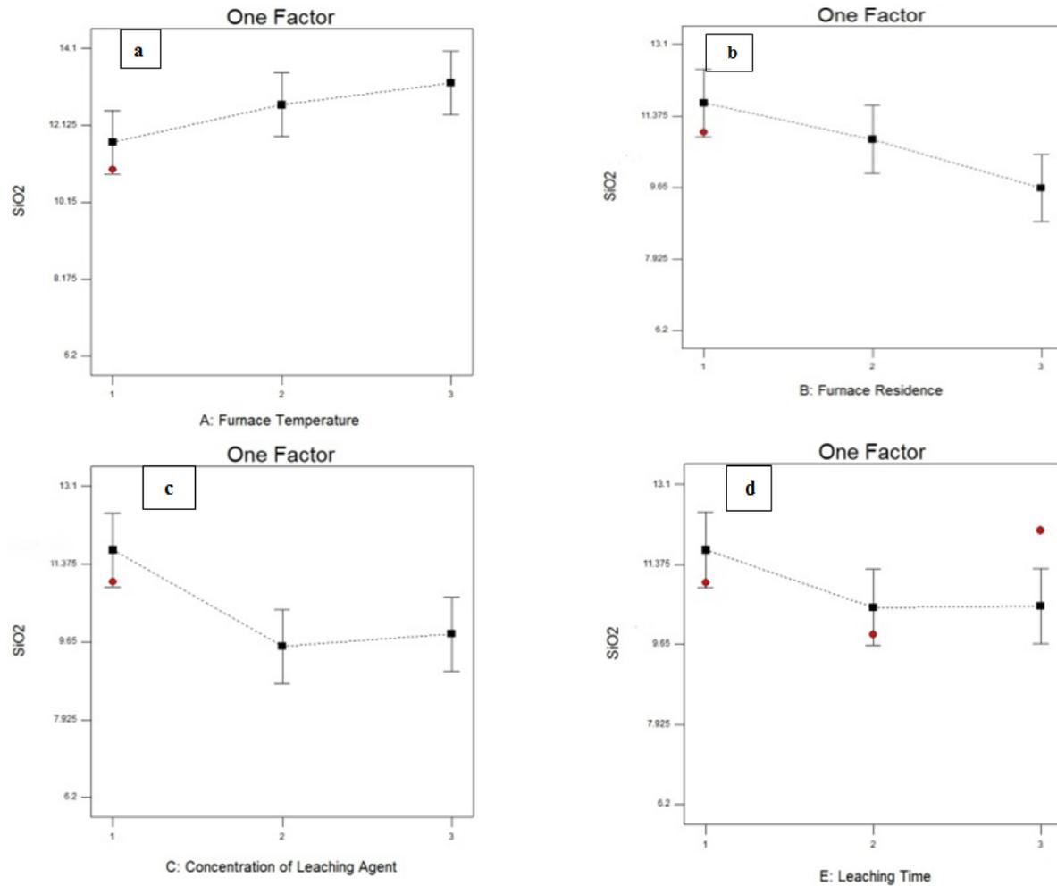
**Figure 4. Trend of SiO<sub>2</sub> content in bauxite vs a) Furnace temperature b) Bauxite residence time in furnace temperature c) Soda concentration d) Leaching time.**
