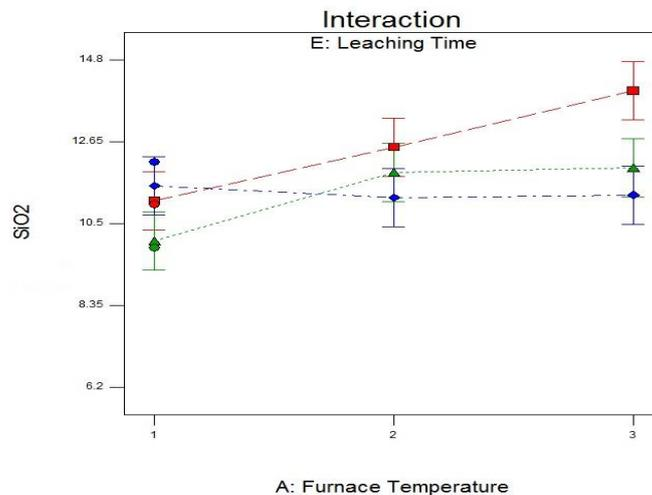
**Figure 2. Interaction between furnace temperature (A) and leaching time (E) for SiO<sub>2</sub> response.**
