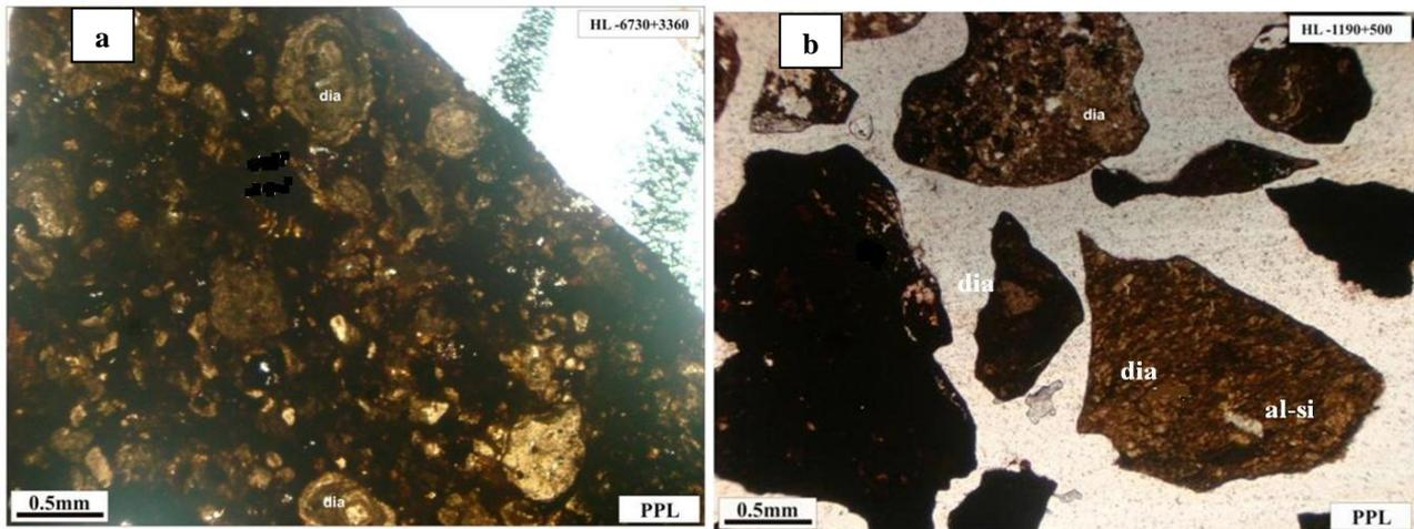
**Figure 1. a) Diaspore (dia) oolitic texture b) Interlocking of diaspora (dia) with aluminosilicates (Al-Si).**
