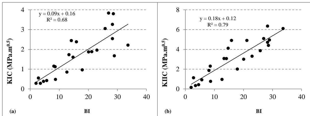
Figure 8. Variation in (a) mode I and (b) mode II fracture toughness with the suggested brittleness index.
