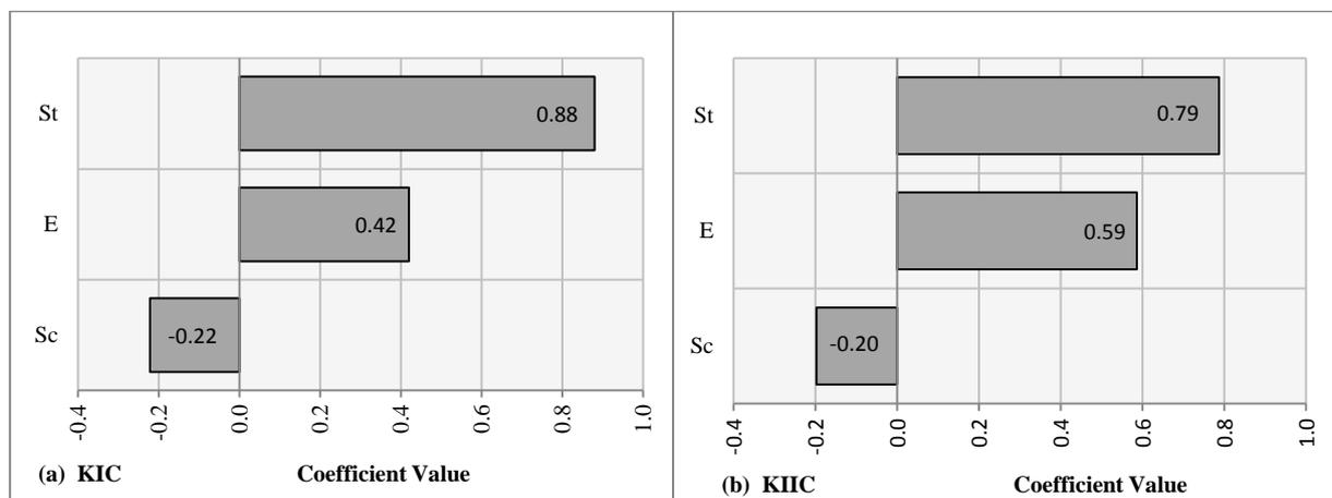
**Figure 7.** Impacts of input parameters of probabilistic analysis on (a)  $K_{IC}$  and (b)  $K_{IIC}$ .
