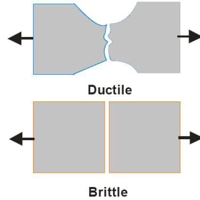
**Figure 2. Brittle and ductile fracturings.**
