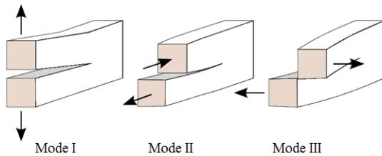
**Figure 1. Three fundamental modes of crack propagation: mode I (tensile), mode II (in-plane shear), and mode III (anti-plane shear).**
