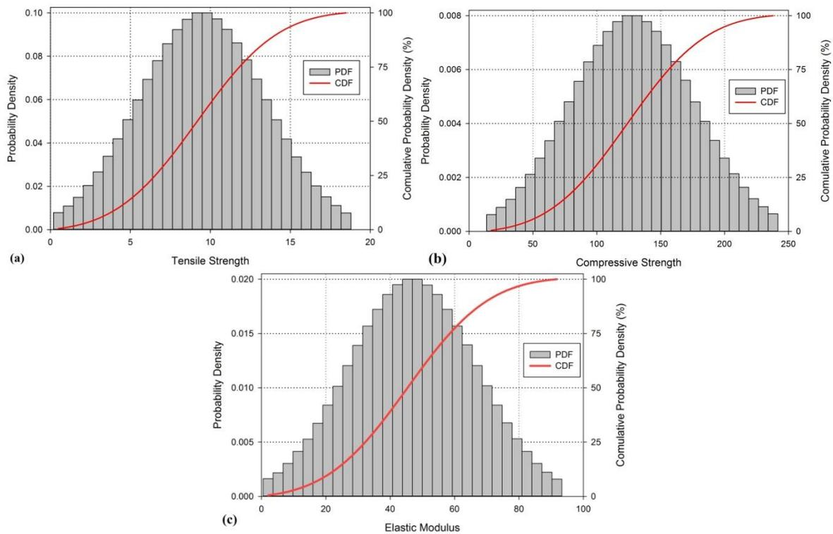
**Figure 6.** PDF and CDF of input parameters (a) tensile strength, (b) compressive strength, and (c) elastic modulus.
