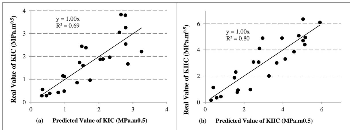
Figure 5. Comparison between real and predicted values for (a)  $K_{IC}$  by Eq. (5), and (b)  $K_{IIC}$  by Eq. (6).
