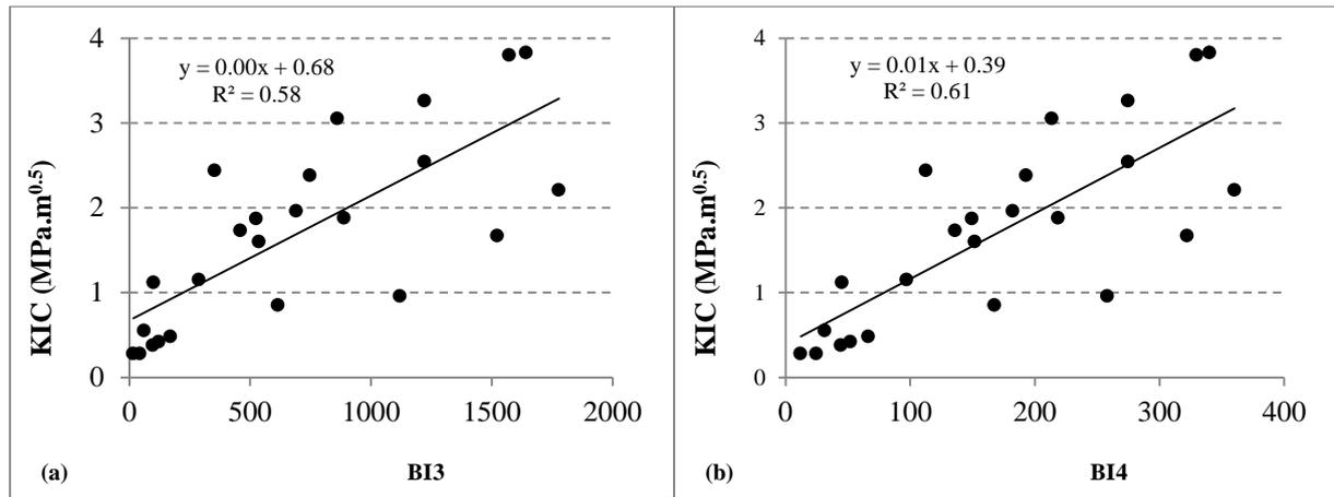
Figure 4. Variation in  $K_{IC}$  with (a)  $BI_3$ , and (b)  $BI_4$ .
