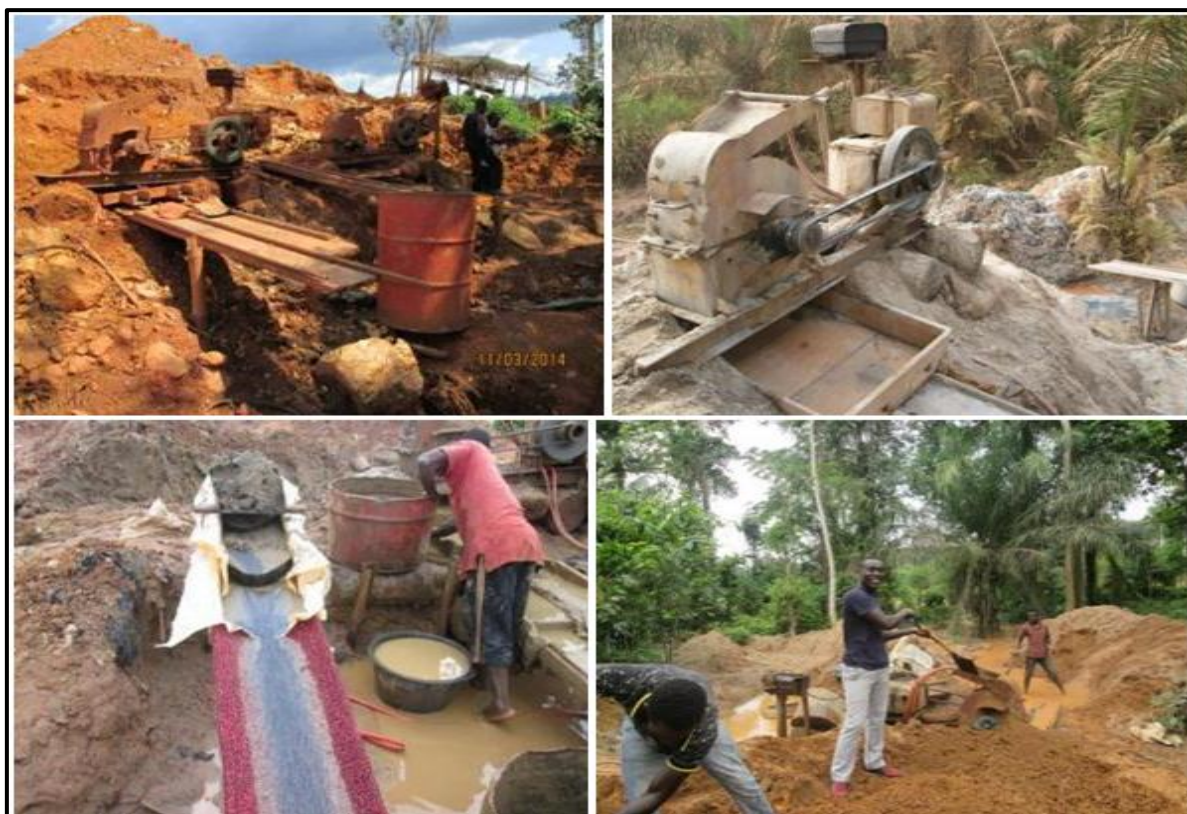
Figure 13. Sluice box fed with “black” (left) at a chamfi site (right) at Mpohor.
