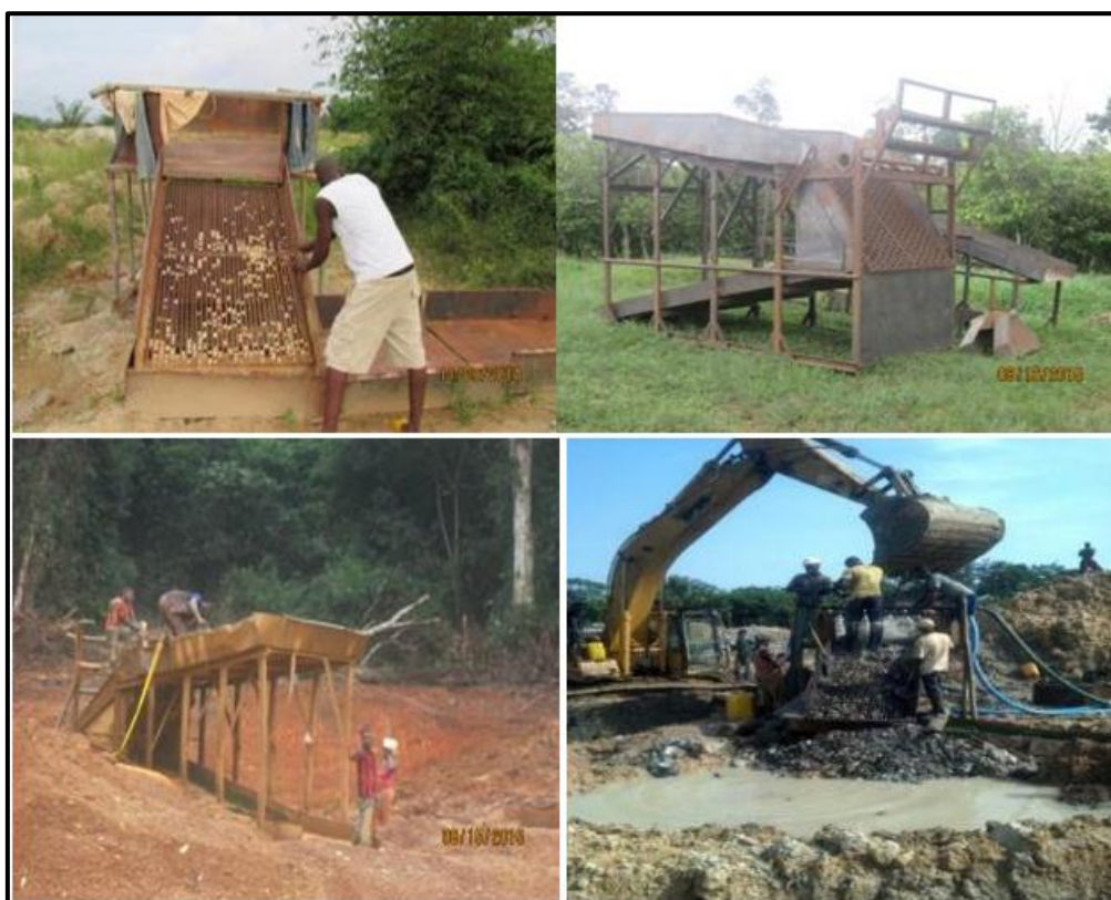
Figure 4. Washing board (coming in different sizes/capacities, configurations, setup, etc.) in operation.
