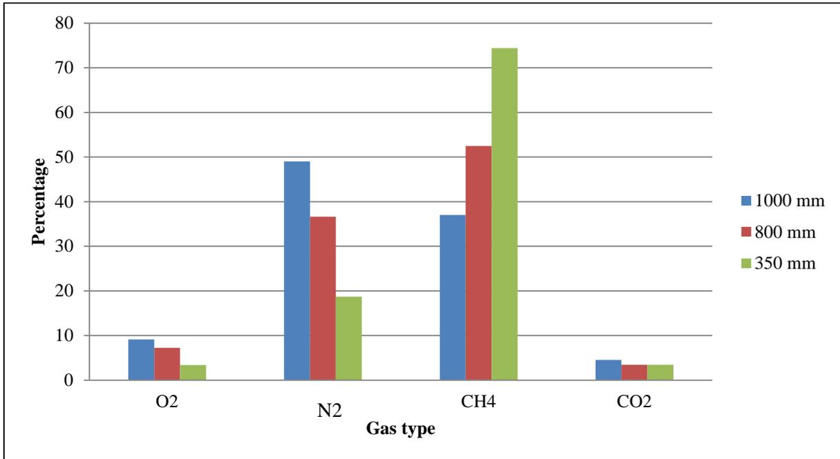
**Figure 3. West Cliff Mine Q2 stage gas component in percentage in coal in different length canisters.**
