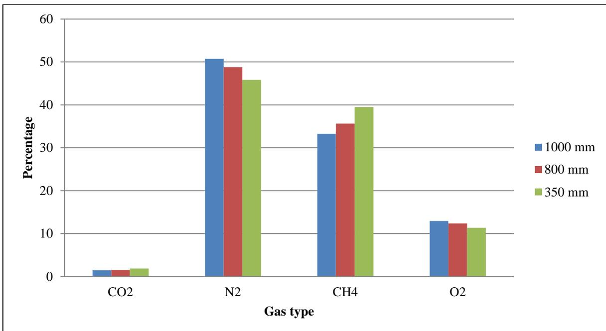
**Figure 4. West Cliff Mine Q3 component percentage analysis from different canisters.**
