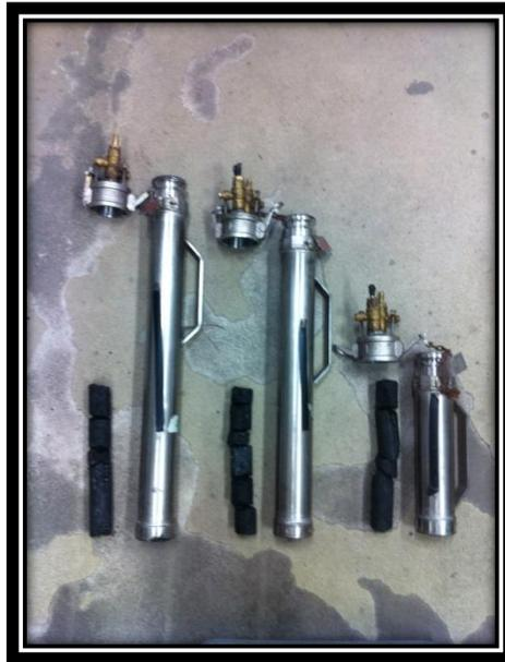
Figure 7. Equal coal column lengths inserted in canisters.
