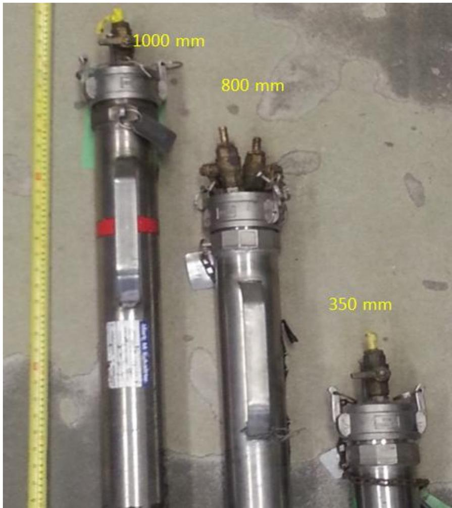
Figure 2. Coal transport canisters of varying lengths.
