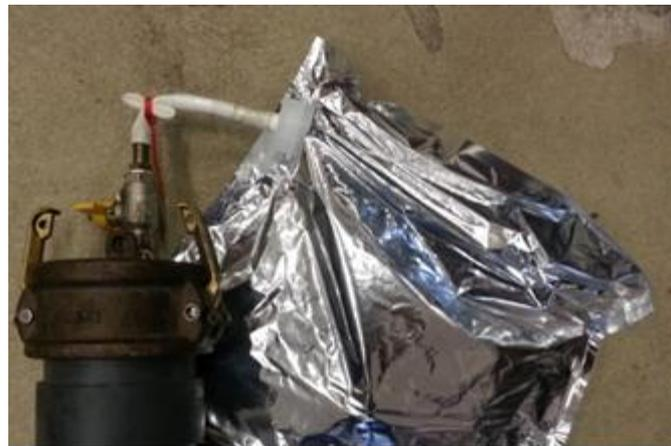
Figure 8. Gas transferred from canister to bags.
