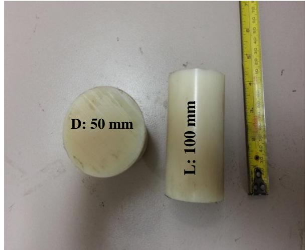
Figure 9b. Resin rods placed in canister A.
