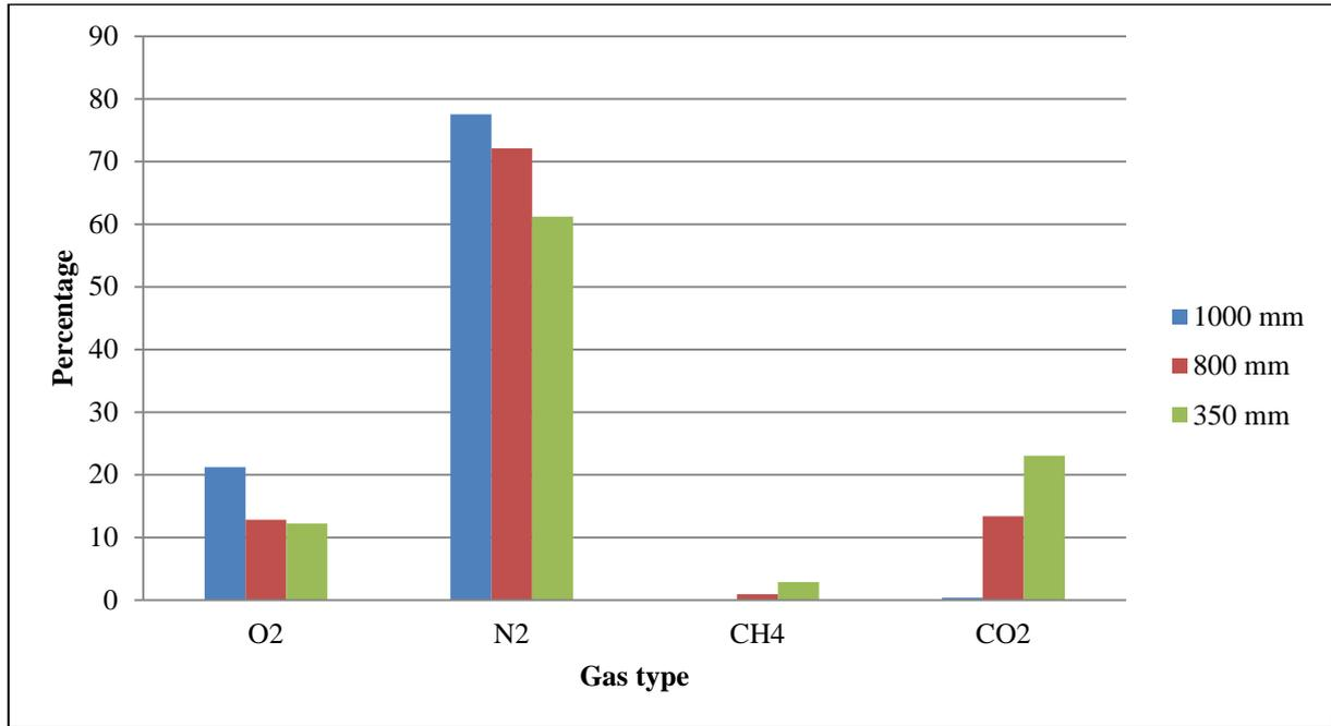
**Figure 5. Tahmoor Mine Q2 gas component percentage analysis from different canisters.**
