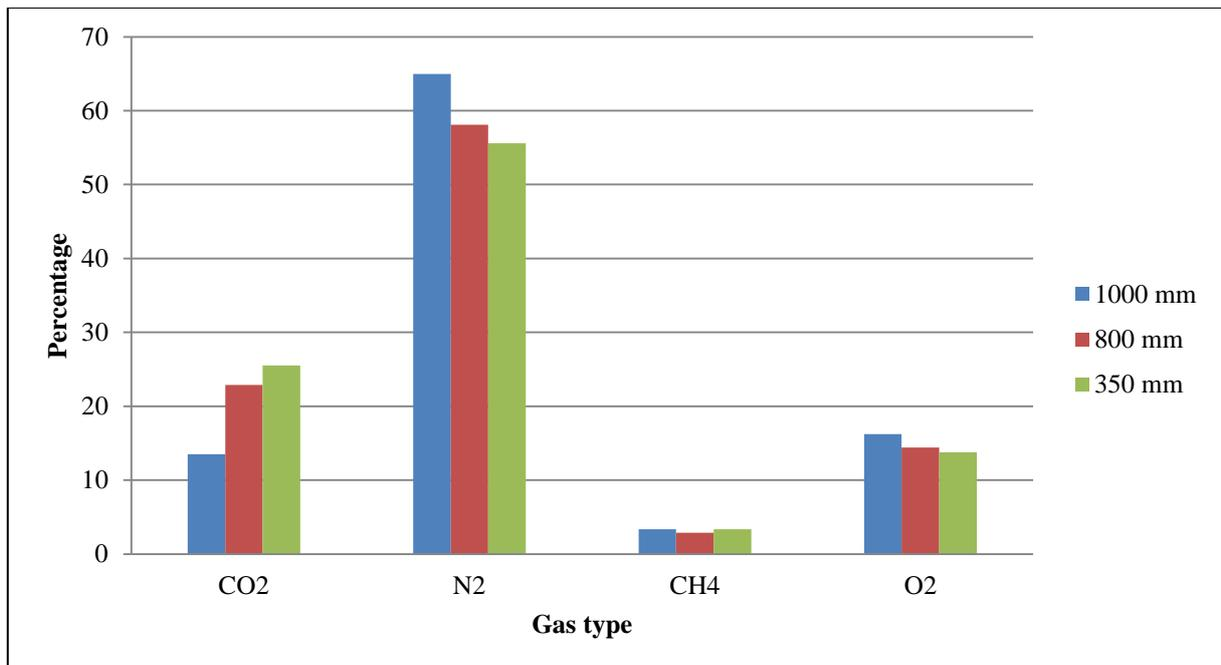
**Figure 6. Tahmoor Q3 component percentage analysis from different canisters.**
