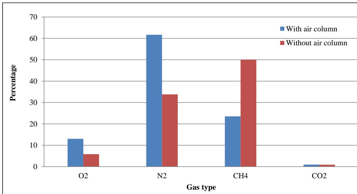
Figure 10. Component percentage with and without trapped air in canisters.
