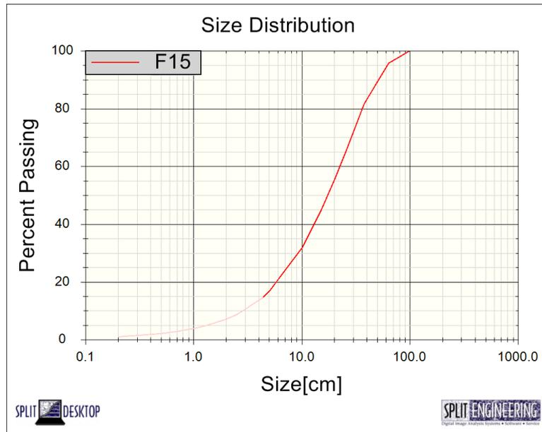
Figure 7. Particle size distribution for fragmented pile in blast no. 16.
