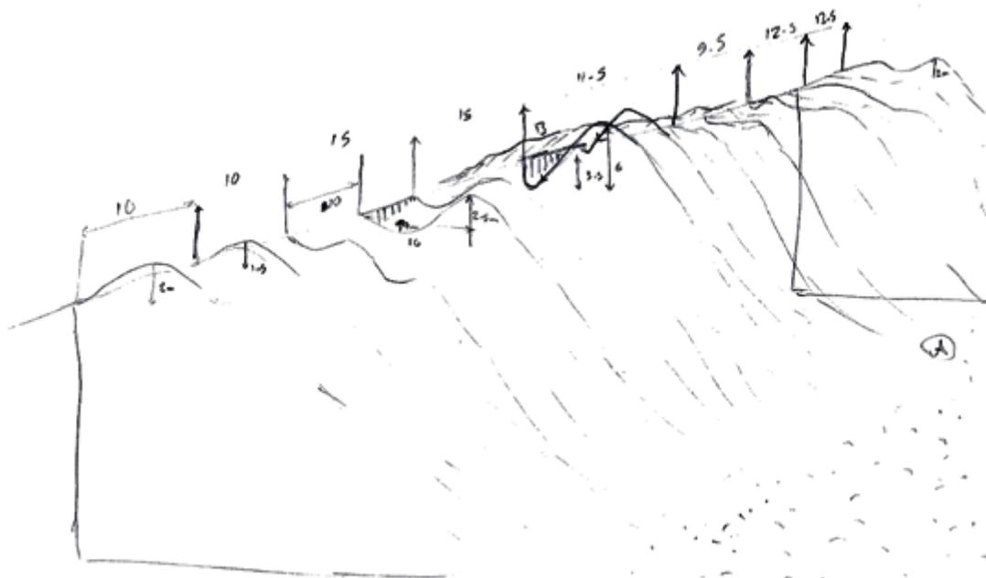
Figure 6. Drawn sections in geodesy of blasted pile in blast no. 12.
