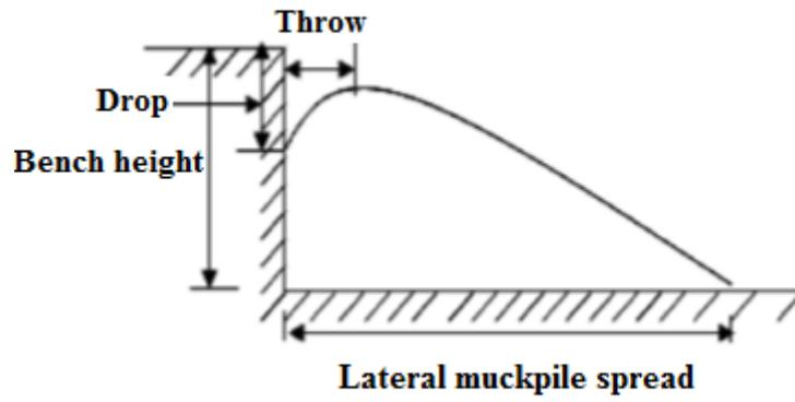
Figure 4. Parameters corresponding to shape of muckpile.
