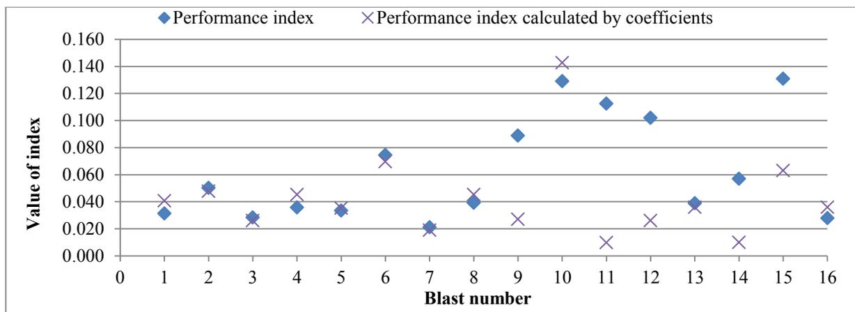
**Figure 11. Comparing real and calculated values of performance indices by applying coefficients.**
