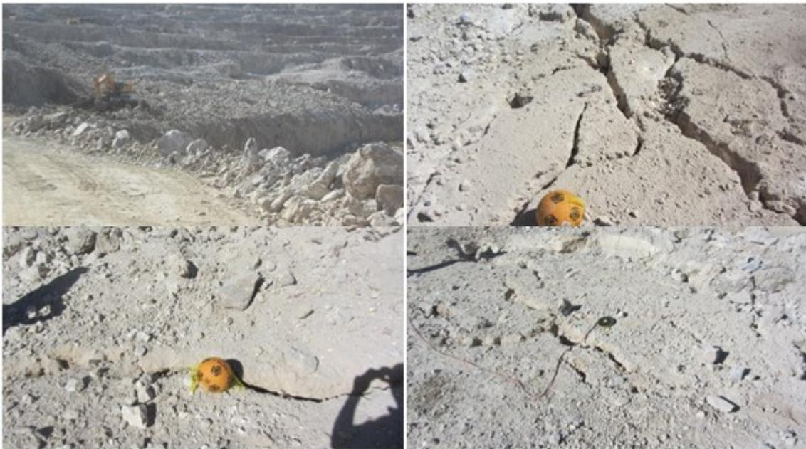
Figure 5. Pile shape and back-break in blast no. 9.
