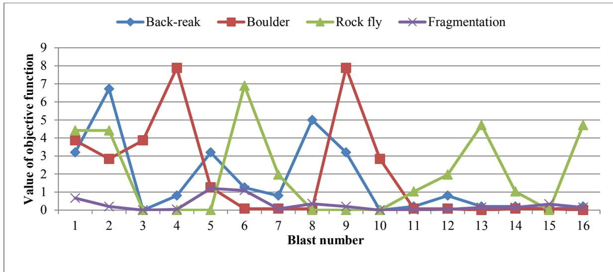
Figure 10. Variations in fragmentation, fly rock, boulder, and back-break in all 16 blasts.
