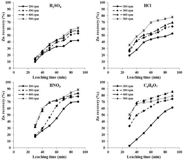
Figure 3. Effect of agitation speed on dissolution of zinc; operation conditions: temperature = 70 °C, L/S ratio = 20 mL/g, HCl concentration = 25%, HNO<sub>3</sub> concentration = 20%, and C<sub>6</sub>H<sub>8</sub>O<sub>7</sub> concentration = 0.75 M.
