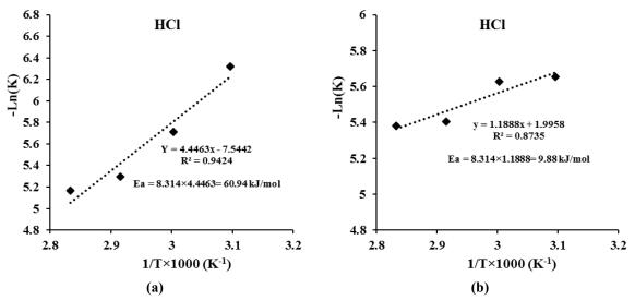
Figure 10. Arrhenius plots for leaching low-grade zinc oxide ore using HCl solution based on surface chemical reaction model in the range of 0-20 min (a) and 20-90 min (b).
