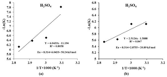
Figure 9. Arrhenius plots for leaching low-grade zinc oxide ore using H<sub>2</sub>SO<sub>4</sub> solution based on surface chemical reaction model in ranges of 0-20 min (a), and 20-90 min (b).
