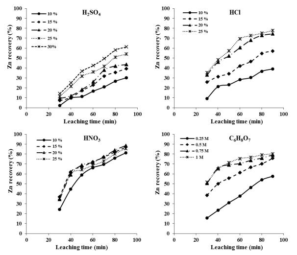
Figure 1. Effect of acid concentrations (H<sub>2</sub>SO<sub>4</sub>, HCl, HNO<sub>3</sub>, C<sub>6</sub>H<sub>8</sub>O<sub>7</sub>) on dissolution of zinc; operation conditions: temperature = 70 °C, L/S = 20 mL/g, agitation speed = 500 rpm.
