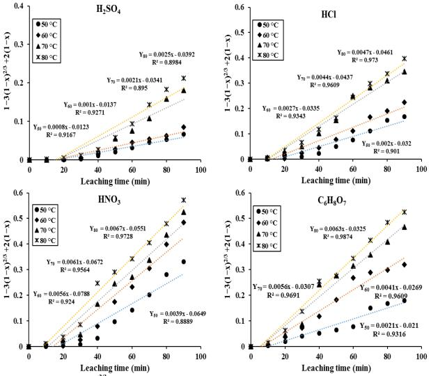
Figure 6. Plot of 1-3(1-x)<sup>2/3</sup>+2(1-x) vs. leaching time at different temperatures for dissolution reactions of zinc with H<sub>2</sub>SO<sub>4</sub>, HCl, HNO<sub>3</sub>, and citric acid solutions.
