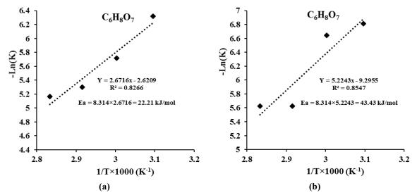
Figure 11. Arrhenius plots for leaching low-grade zinc oxide ore using citric acid solution based on surface chemical reaction model in ranges of 0-70 min (a) and 70-90 min (b).
