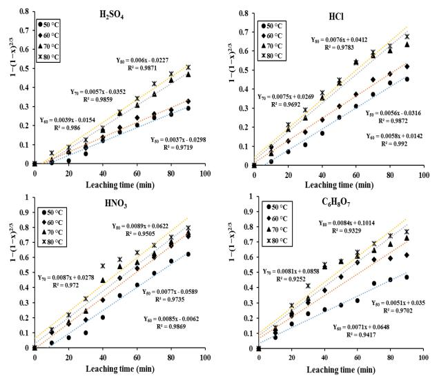
Figure 5. Plot of 1-(1-x)<sup>2/3</sup> vs. leaching time at different temperatures for dissolution reactions of zinc with H<sub>2</sub>SO<sub>4</sub>, HCl, HNO<sub>3</sub>, and citric acid solutions.
