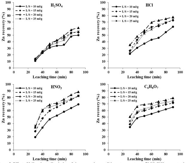
Figure 2. Effect of L/S ratio on dissolution of zinc; operation conditions: temperature = 70 °C, HCl concentration = 25%, HNO<sub>3</sub> concentration = 20%, C<sub>6</sub>H<sub>8</sub>O<sub>7</sub> concentration = 0.75 M, agitation speed = 500 rpm.
