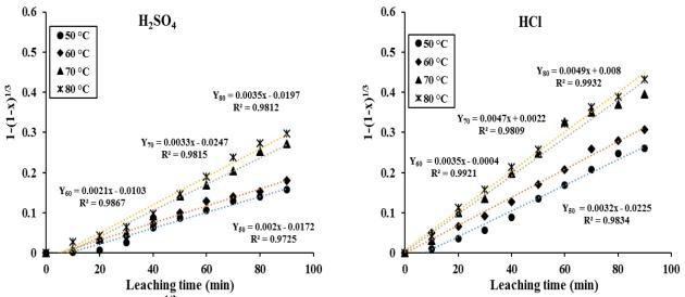
Figure 7. Plot of 1-(1-x)<sup>1/3</sup> vs. leaching time at different temperatures for dissolution reactions of zinc with H<sub>2</sub>SO<sub>4</sub>, HCl, HNO<sub>3</sub>, and citric acid solutions.
