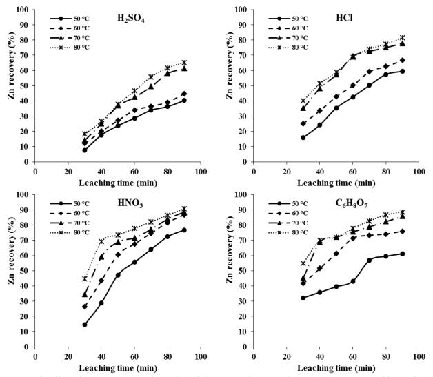
Figure 4. Effect of temperature on dissolution of zinc; operation conditions: agitation speed = 500 rpm for inorganic acids and 400 rpm for citric acid, L/S ratio = 20 mL/g; HCl concentration = 25%, HNO<sub>3</sub> concentration = 20%, and  $C_6H_8O_7$  concentration = 0.75 M.
