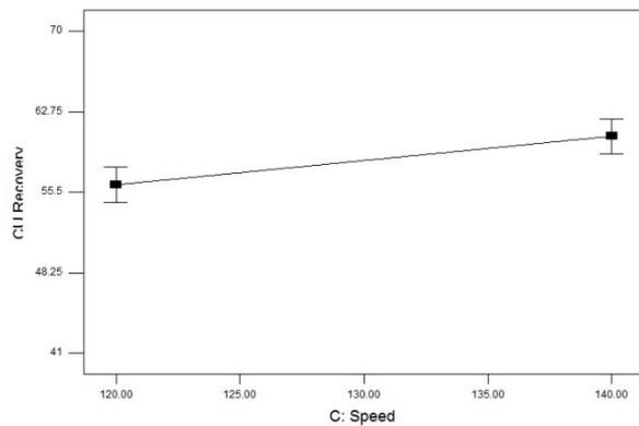
Figure 14. Cu recovery for various speeds of shaking.
