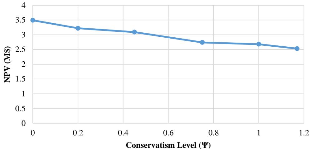
Figure 6. NPV versus different counterpart optimization level, objective function uncertainty, and RHS+LHS uncertainty for all constraints (Marvin 3D orebody).
