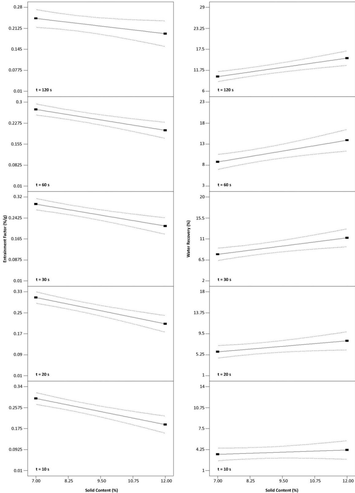
Figure 3. Effects of solid content on entrainment factor and water recovery.
