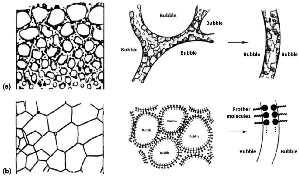
Figure 8. Comparison between stabilization mechanism in froth (a) and foam (b) phases ([38], modified).
