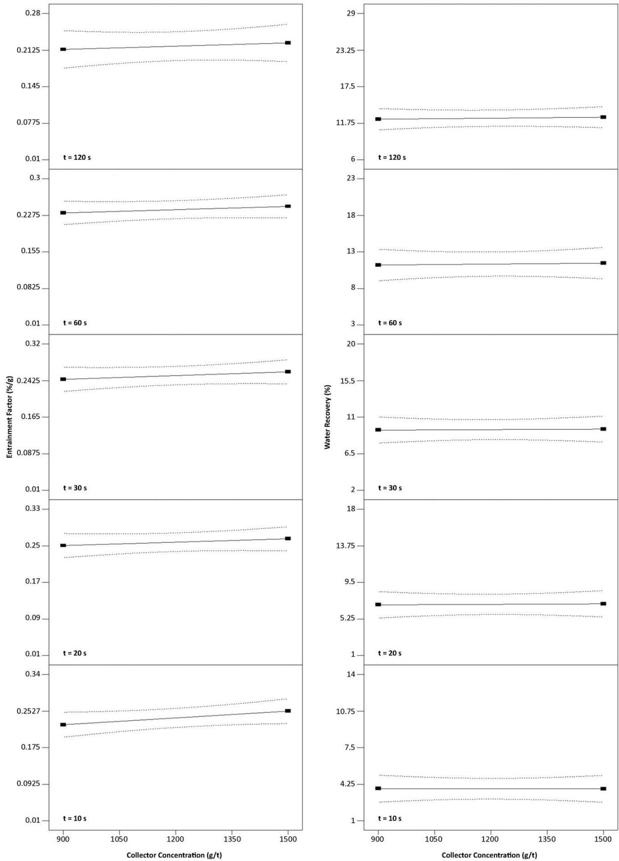
Figure 5. Effect of collector concentration on entrainment factor and water recovery.
