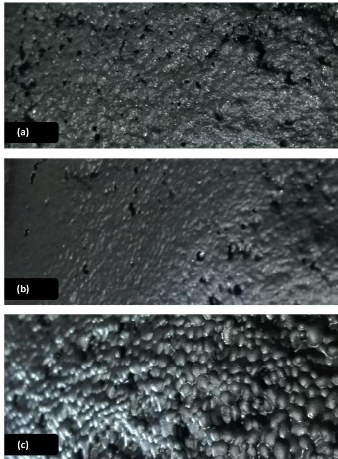
**Figure 14.** Effect of particle size on froth structure before about 30 s of flotation: (a) +150-500  $\mu\text{m}$ , (b) +45-150  $\mu\text{m}$ , and (c) -45  $\mu\text{m}$ .
