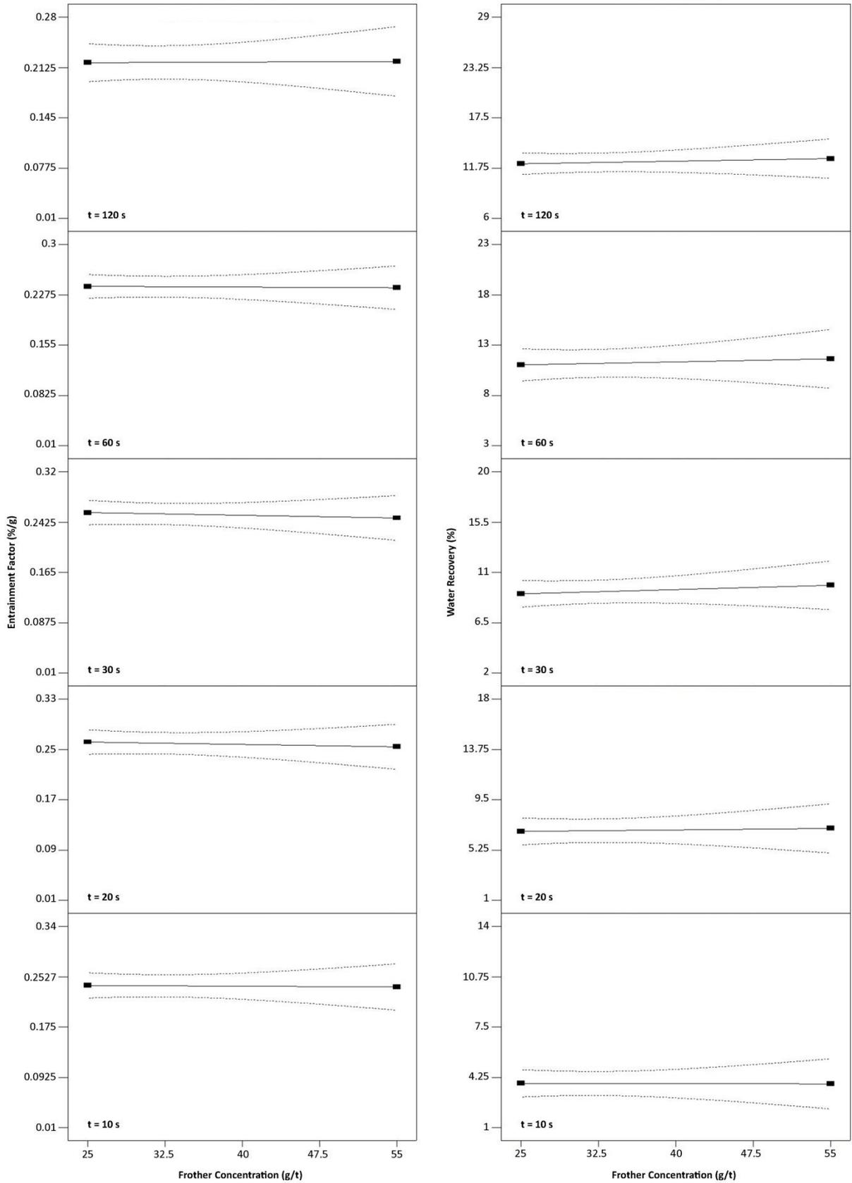
Figure 7. Effects of frother concentration on entrainment factor and water recovery.
