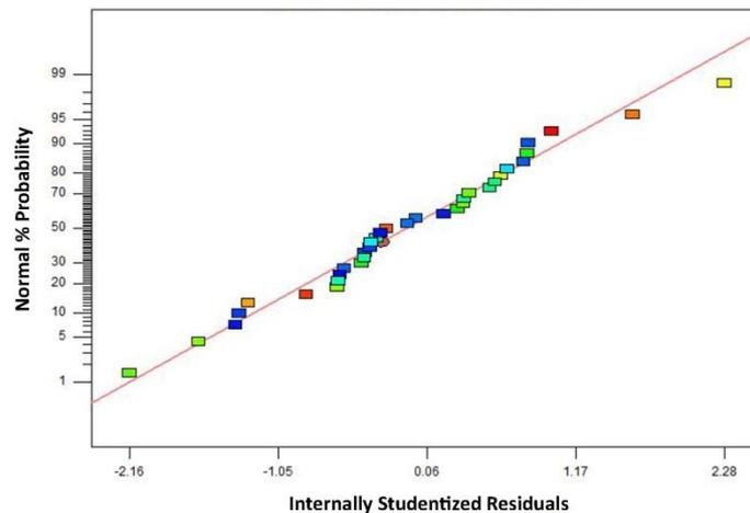
Figure 1. Normal Probability plot of residuals for entrainment factor after 10 s of flotation.
