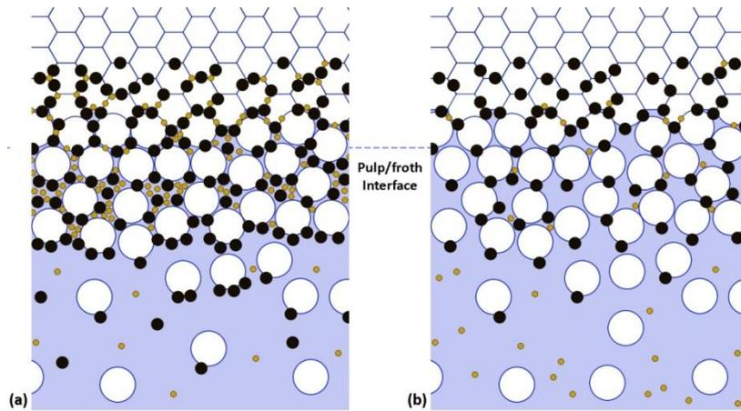
Figure 12. Schematic illustration of swarm theory in coarse particle flotation as proposed in this study: (a) before 30 s, and (b) after 30 s.
