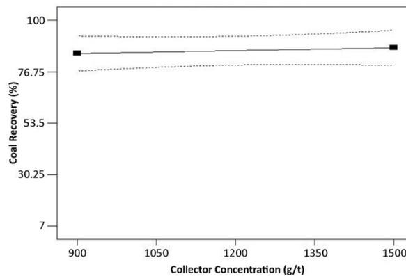
Figure 6. Effect of collector concentration on final coal recovery.
