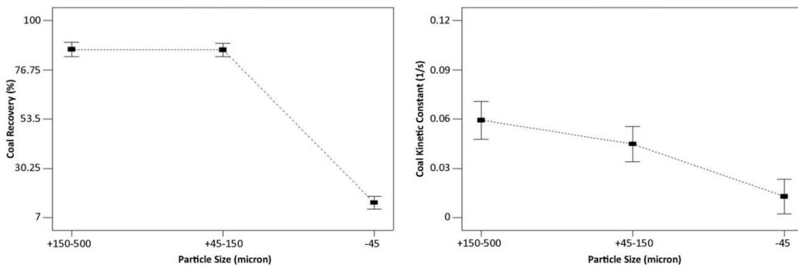
**Figure 4. Effect of particle size on coal recovery and kinetic rate.**
