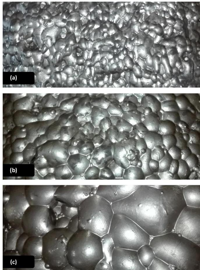
Figure 9. Change in structure of froth during coal flotation test after (a) 30 s, (b) 60 s, and (c) 120 s.
