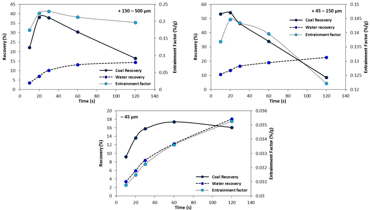
Figure 13. Time-step plots of coal recovery, entrainment factor, and water recovery for different particle size fractions.
