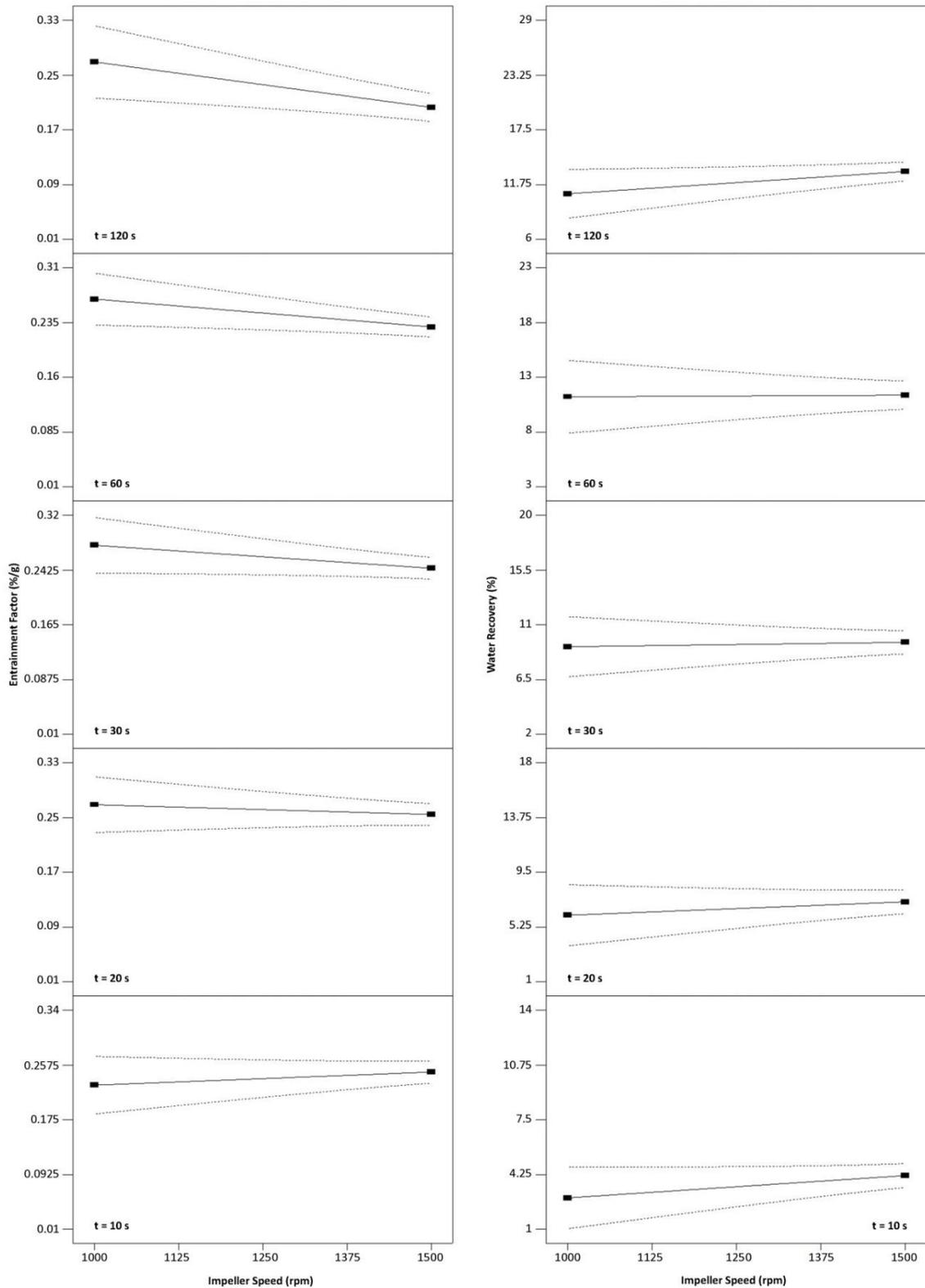
Figure 10. Effect of impeller speed on entrainment factor and water recovery.
