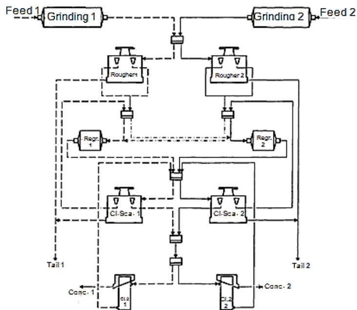
Figure 4. Equipment layout of the Sarcheshmeh concentrator No. 2.
