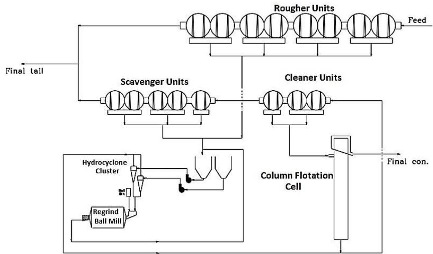
Figure 2. Flotation circuit of the Sarcheshmeh concentrator No. 2 [1].
