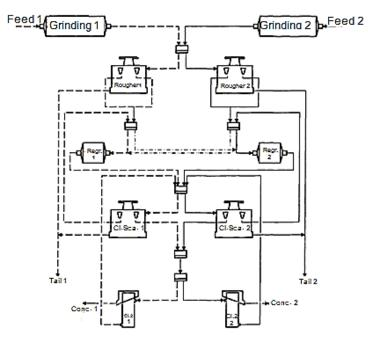
Figure 4. Equipment layout of the Sarcheshmeh concentrator No. 2.
