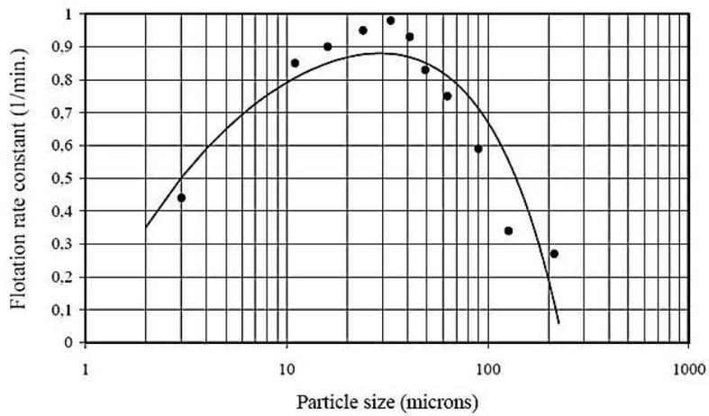
Figure 3. Variation in flotation rate constant with particle size [3].
