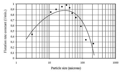
Figure 3. Variation in flotation rate constant with particle size [3].
