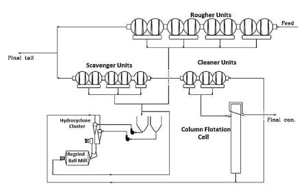
Figure 2. Flotation circuit of the Sarcheshmeh concentrator No. 2 [1].
