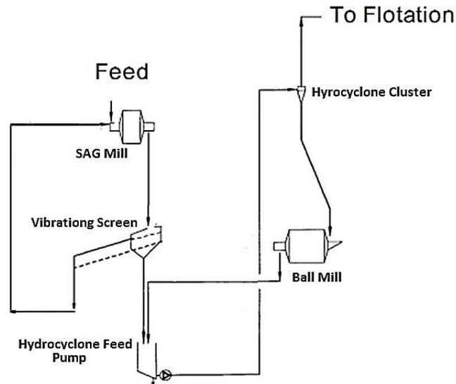
Figure 1. Grinding circuit of plant No. 2 of the Sarcheshmeh copper complex [1].
