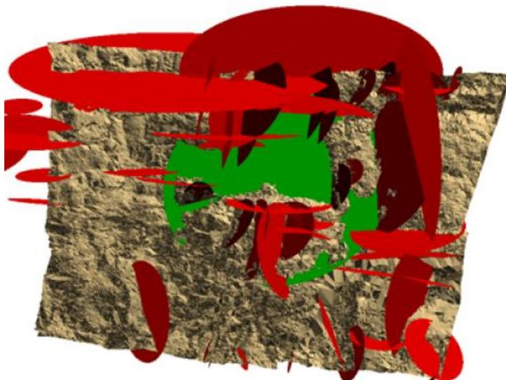
Figure 7. Recording discontinuities observed through sampling window.
