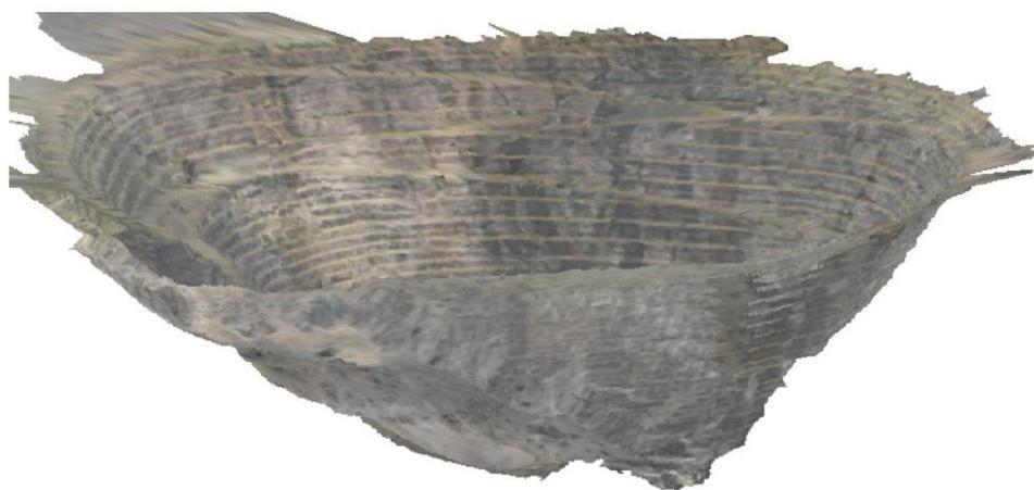
Figure 4. A stereomodel of pit mine using photogrammetric images ( $f = 100$  mm).
