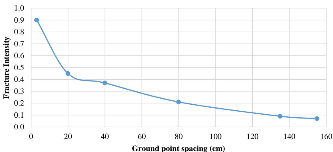
Figure 10. Variation trend of areal fracture intensity with ground point spacing.
