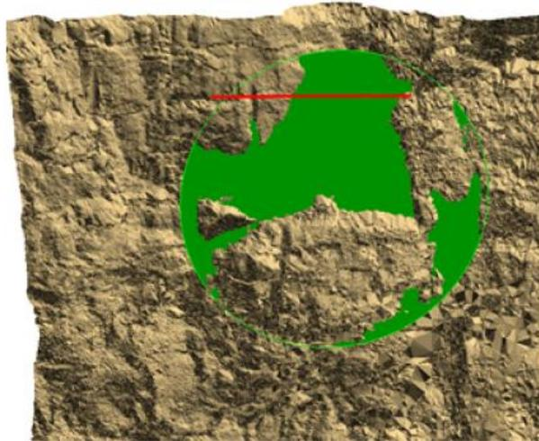
Figure 6. Defining a circular sampling window with a diameter of 10 m.
