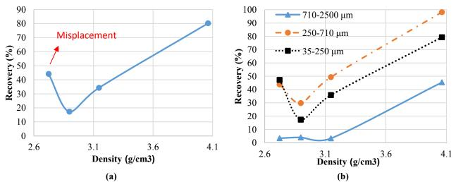
Figure 3. (a) Partition curve of DTP spiral circuit. (b) Size-by-size partition curve of DTP spiral circuit.
