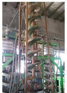
Figure 2. Pilot-plant spiral installed in a closed continuous system.
