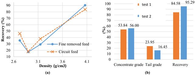
Figure 4. (a) Simulation of fine particle removal effect on DTP spiral circuit partition curve. (b) Iron recovery and grade of two pilot-scale tests (test 1: original sample, test 2: fines removed from sample).
