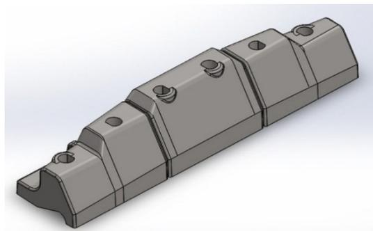
Figure 13. 3D model of second non-uniform liner (design No. 3).
