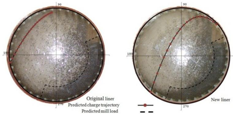
Figure 6. Charge shape and trajectory of original and new liners in laboratory mill (20% filling).
