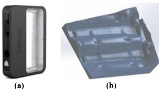
Figure 3. a) 3D scanner (Sense<sup>®</sup>) used in this research work, b) a typical snapshot of a scanned liner.
