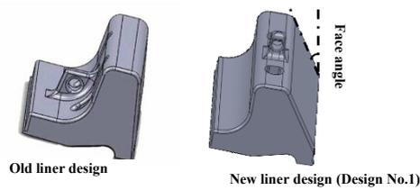
Figure 7. 3D model of original and new liners used at Gol-E-Gohar concentration plant mills.
