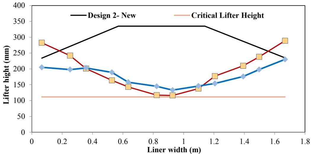
Figure 12. Variations in maximum lifter heights along mill length for uniform and non-uniform liners after 6200 h of operation.
