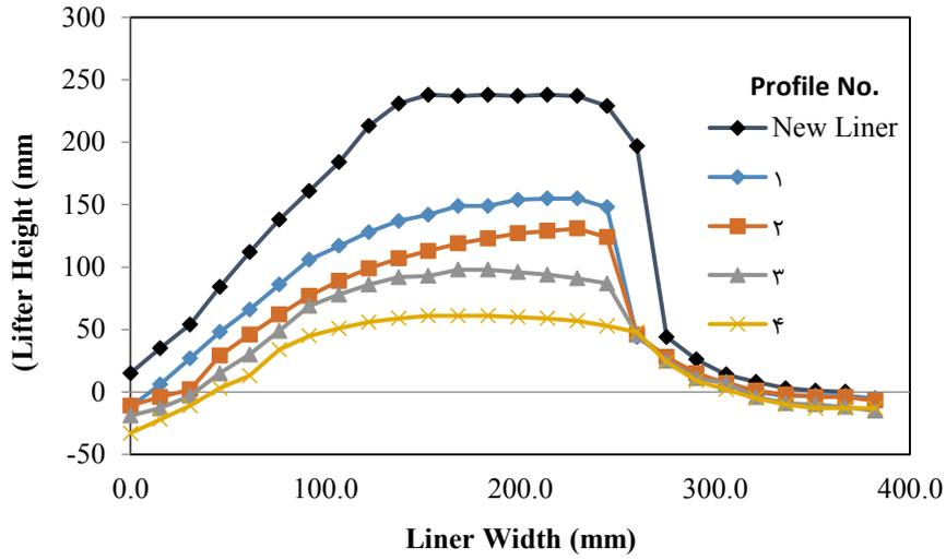
Figure 8. Wear profiles of a liner after 6200 h of operation at four points along length of liner.
