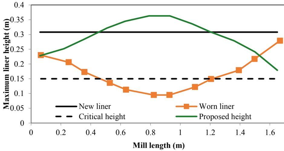
Figure 9. Variations in maximum lifter heights along liner after 6200 h of operation.
