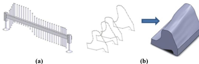
Figure 2. a) Pin gauge, b) typical 3D model of a worn liner after 3000 h of operation at Gol-E-Gohar concentration plant.
