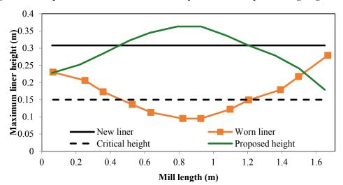
Figure 9. Variations in maximum lifter heights along liner after 6200 h of operation.
