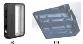
Figure 3. a) 3D scanner (Sense<sup>©</sup>) used in this research work, b) a typical snapshot of a scanned liner.
