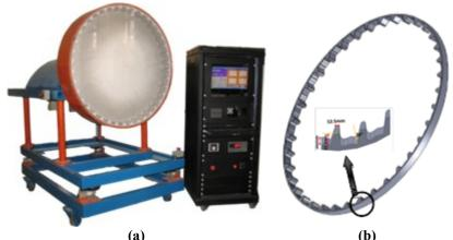
Figure 1. a) Model mill along with control and data acquisition system, b) polyurethane ring machined to scale down liners arrangement of an industrial mill.
