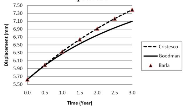
**Figure 4. Comparison of wall displacement of lined tunnel**
