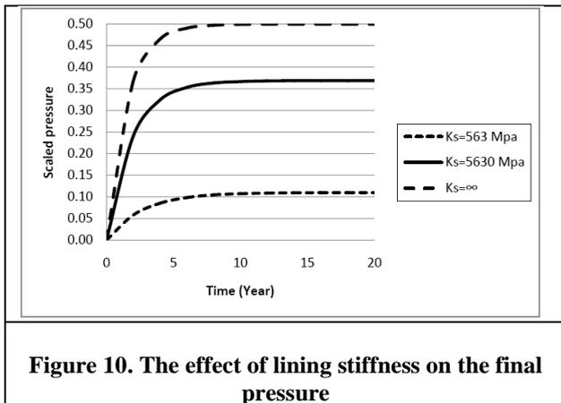
**Figure 10. The effect of lining stiffness on the final pressure**
