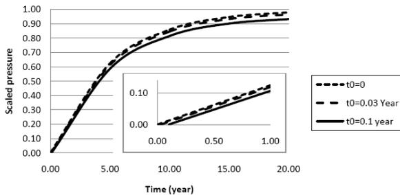
Figure 6. The effect of different delay time on lining pressure
