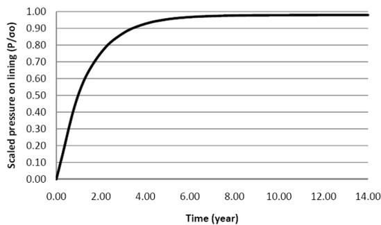
**Figure 2. Scaled pressure on lining**
