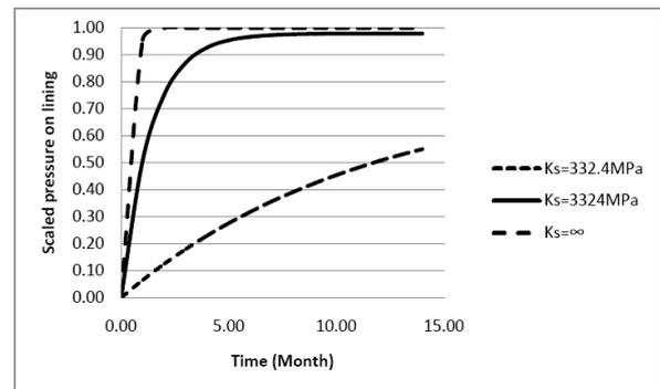
**Figure 3. Effect of lining stiffness on applied pressure**
