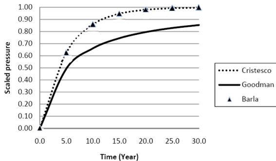
Figure 5. Comparison of scaled pressure on the tunnel lining
