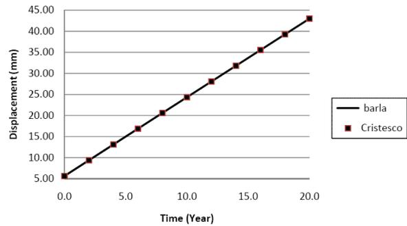
Figure 7. Creep displacement of tunnel wall
