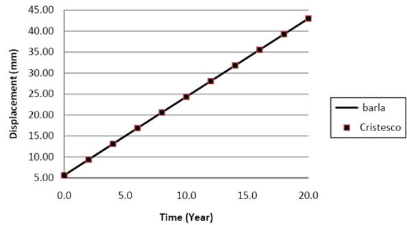
Figure 7. Creep displacement of tunnel wall
