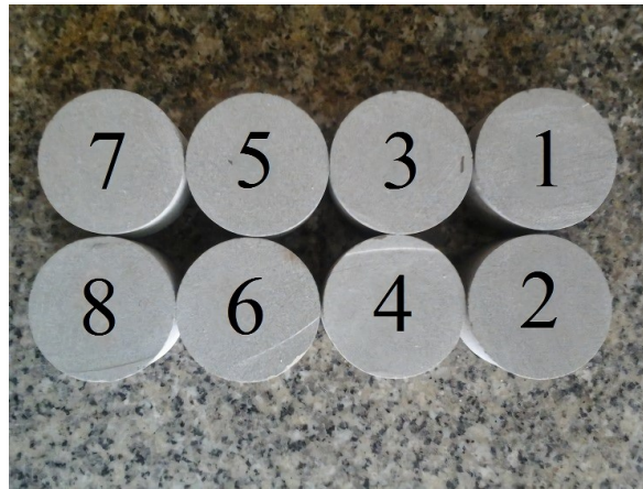
Figure 6. Sandstone disc samples for Brazilian test.
