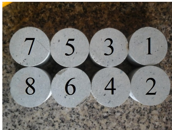
Figure 7. Tuff disc samples for Brazilian test.
