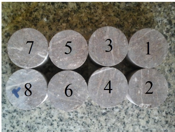
Figure 8. Andesite disc samples for Brazilian test.
