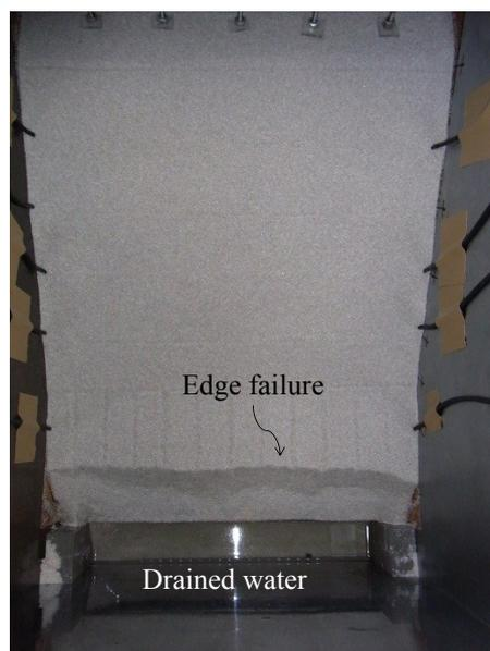
**Figure 14. Water drainage from Silica sand. No. 6 model during g-up process.**
