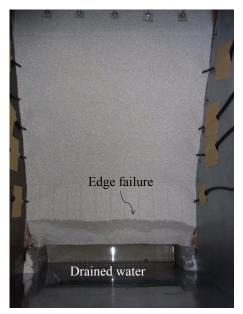
Figure 14. Water drainage from Silica sand. No. 6 model during g-up process.
