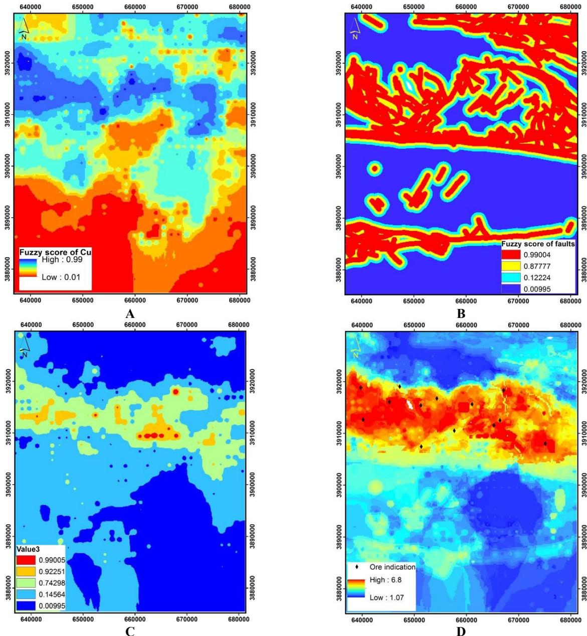
Figure 10. Fuzzy evidence layer of (A) Cu geochemical signature, (B) fault density, (C) Zn geochemical signature (D) fuzzy prospectivity model generated by integration evidence layers.
