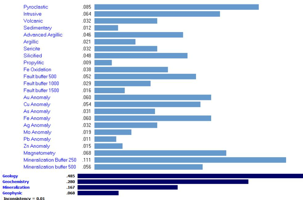
**Figure 12. Parameter weighting of different data and structure layer based on AHP with inconsistency = 0.01.**
