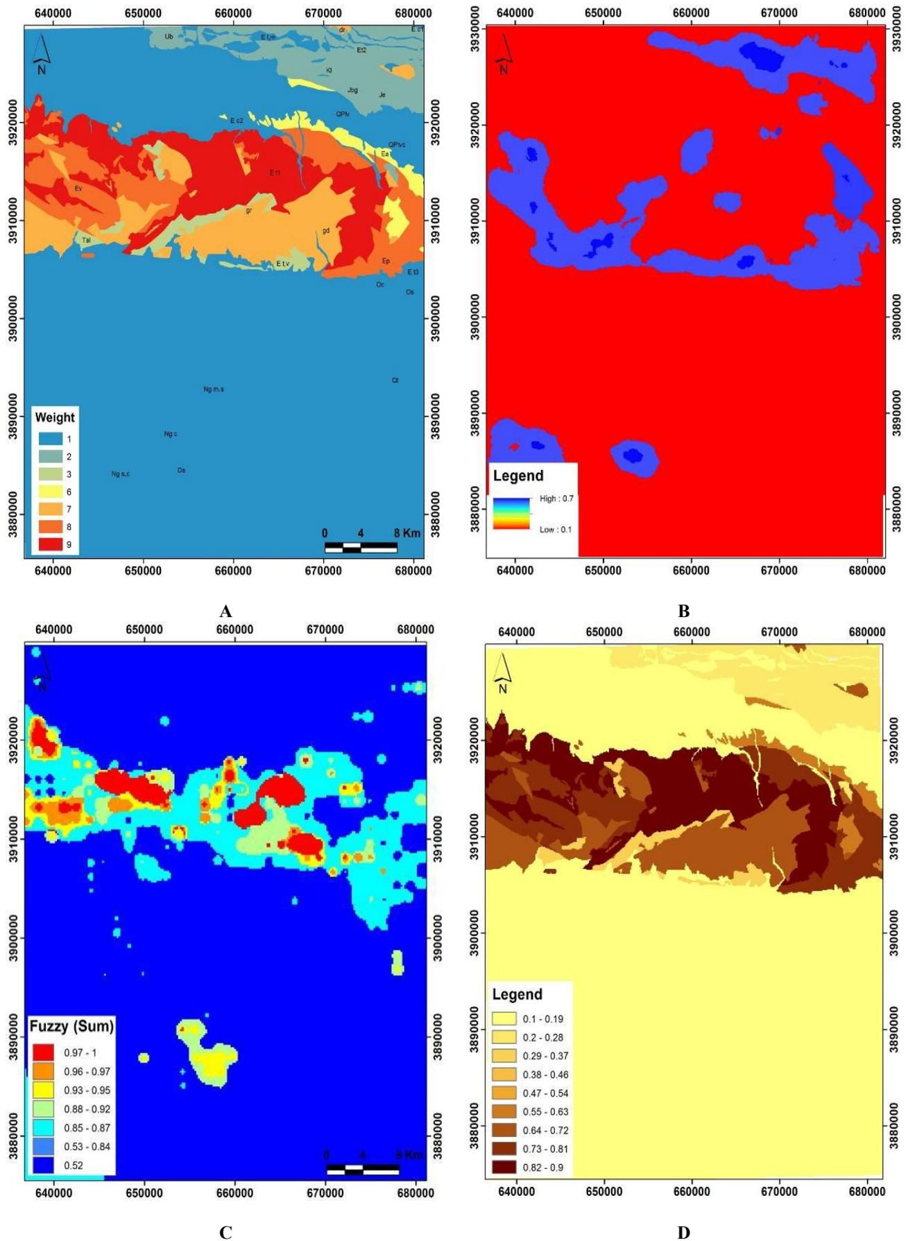
Figure 8. Some weighted evidential layers: A) geology (for AHP) B) fault intersection (for fuzzy) C) geochemistry (fuzzy sum operator) D) geology (fuzzy).
