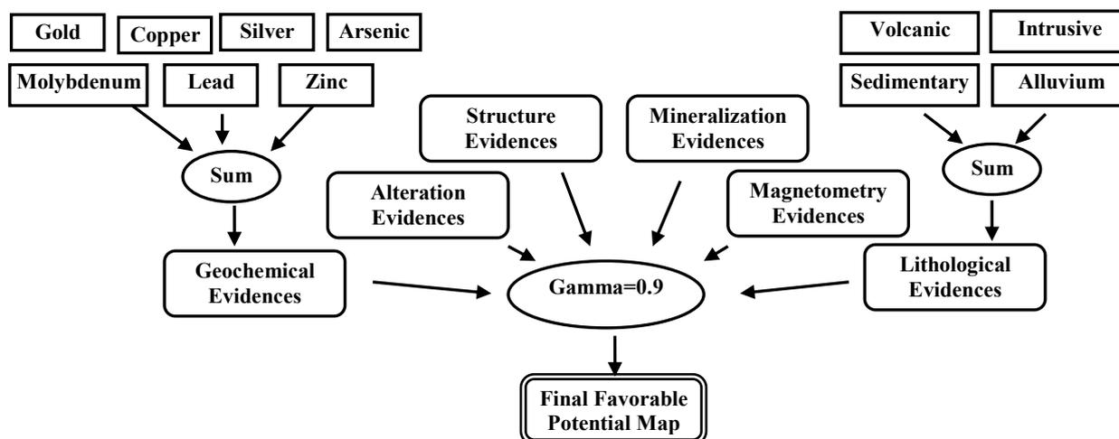
**Figure 9. Schematic inference network for MPM in Feyz-Abad area.**
