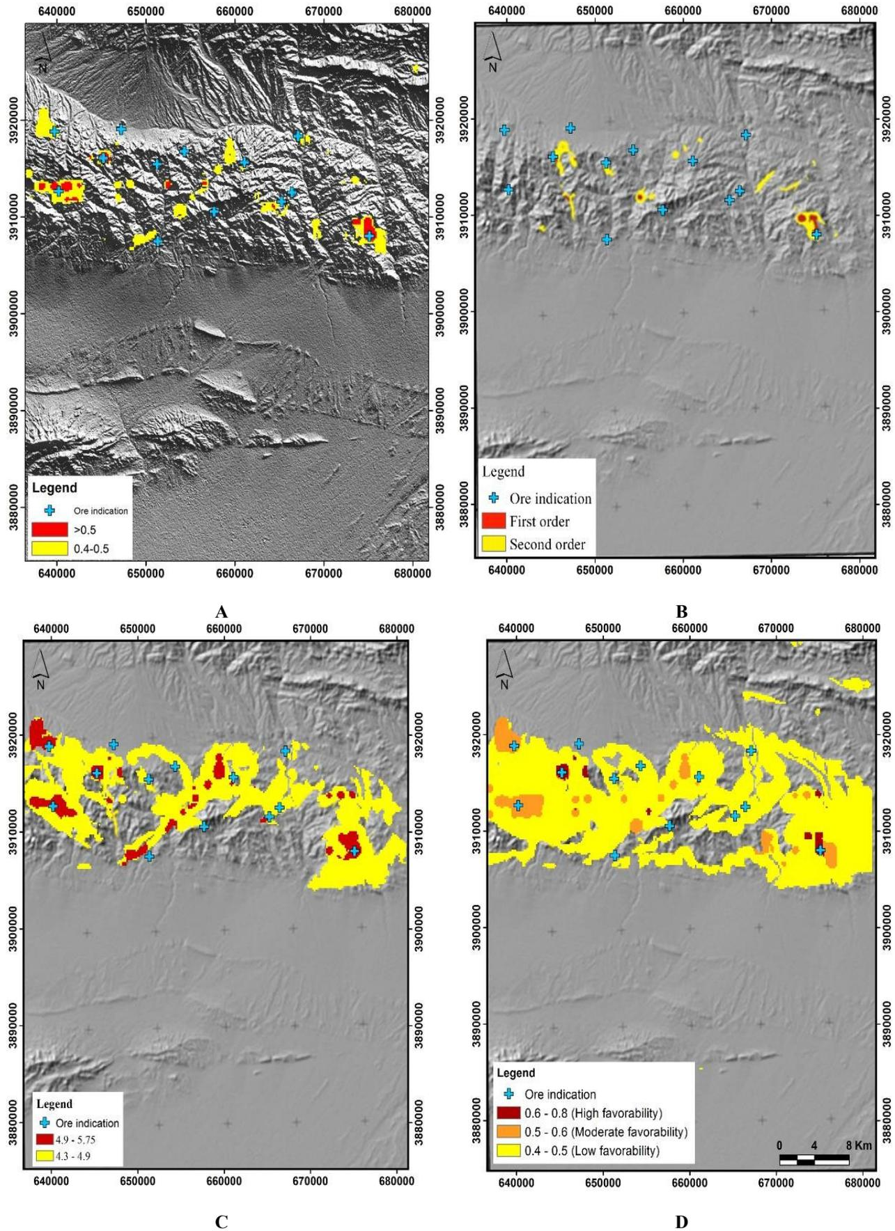
Figure 14. Promising areas for MPM in Feyz-Abad area based on a) fuzzy method, b) index overlay integration, c) AHP method, and d) Fuzzy AHP.
