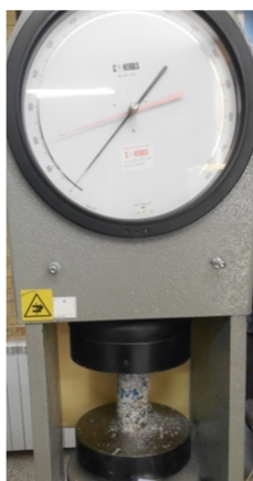
Figure 4. Uniaxial compressive strength test.
