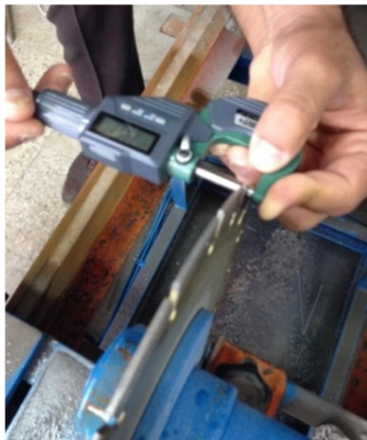
Figure 6. Digital micrometer for measuring saw wear.
