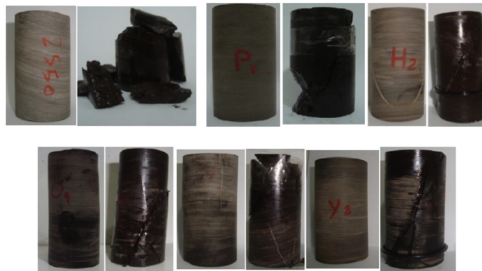
Figure 3. Samples before and after multi-stage triaxial test.
