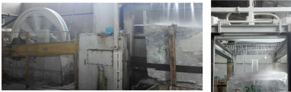
Figure 1. Gang saw machine used in this case.
