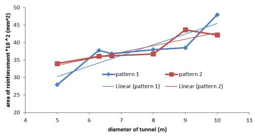
Figure 13. Effect of joint arrangement patterns on area of steel reinforcement.
