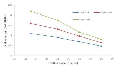
Figure 16. Effect of internal friction angle on optimal cost of segmental lining.
