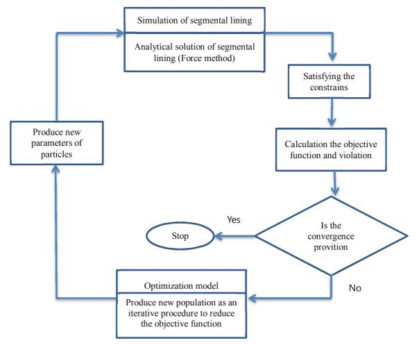
Fig 5. Combination process of simulation and optimization algorithms.
