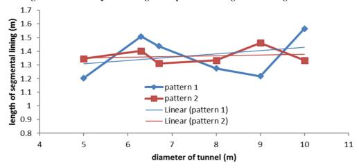
Figure 12. Effect of joint arrangement patterns on segmental lining length.
