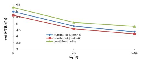
Figure 9. Effect of number of lining joints on objective function changes.
