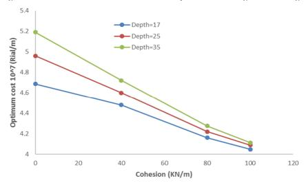
Figure 15. Effect of soil cohesion on optimal cost of segmental lining.
