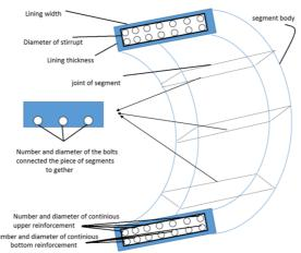
Figure 1. Schematic view of design variables.
