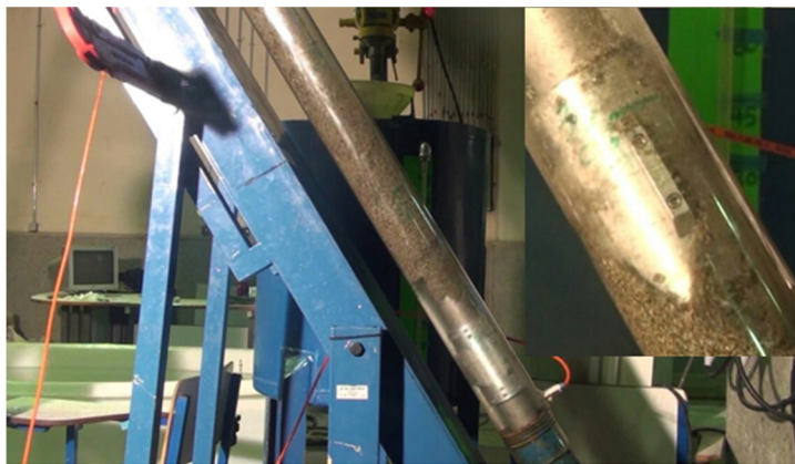
Figure 10. A simplified stabilizer is located at two specific distances of 8 cm of the drill bit.
