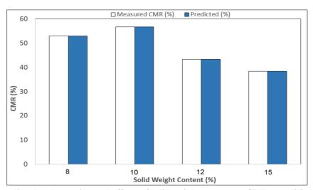
Figure 17. The predicted and experimental effects of solid weight content on CMR: conditioning time, 3 min; rotor speed, 1200 RPM; pH, 8; flotation retention time, 3 min; collector dosage, 250 g/ton; frother dosage, 50g/ton; and feed ash, 41.9%.
