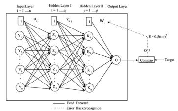
Figure 1. A flowchart of a typical two-hidden-layer BPNN [23].
