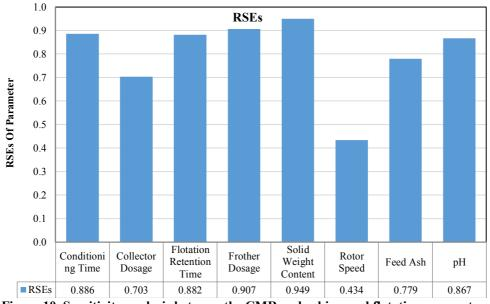
Figure 10. Sensitivity analysis between the CMR and coking coal flotation parameters.
