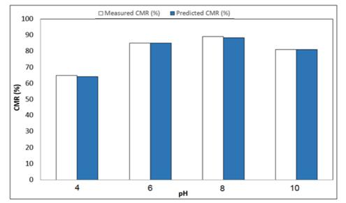
Figure 11. The predicted and experimental effects of pH on CMR: conditioning time, 3min; gasoline dosage, 500 g/ton; flotation retention time, 3 min; MIBC dosage, 50 g/ton; solid weight content, 12%; rotor speed, 1200 RPM; and feed ash, 43.5%.
