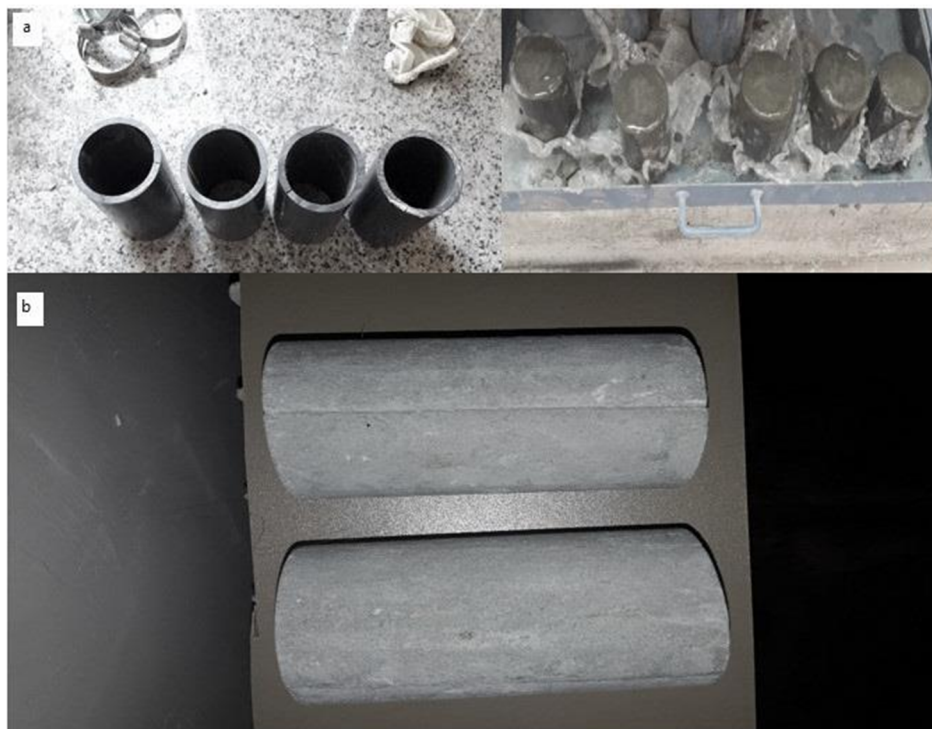
Figure 1. (a) PVC pipes for preparation of specimens; (b) specimens prepared for determination of physical and mechanical properties.
