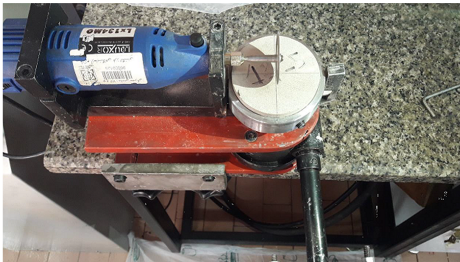
Figure 6. A finger milling with a special base to create a chevron notch.
