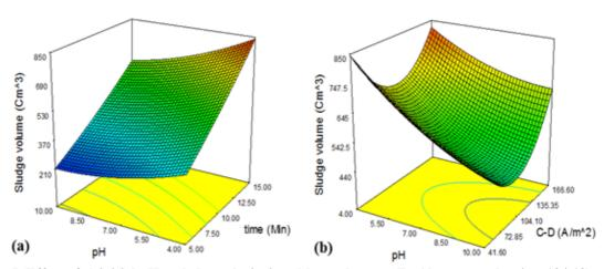
Figure 5. Effect of a) initial pH and electrolysis time (electrode type: Fe-Al; current density: 104.10), and b) initial pH and current density (electrode type: Fe-Al; electrolysis time: 10 min) on sludge volume (Cm3); 3D surface plots.
