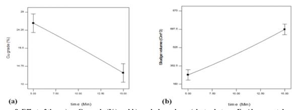
Figure 8. Effect of time a) on Cu grade (%) and b) on sludge volume (electrode type: Fe-Al; current density: 104.10; initial pH: 7), One factor plot
