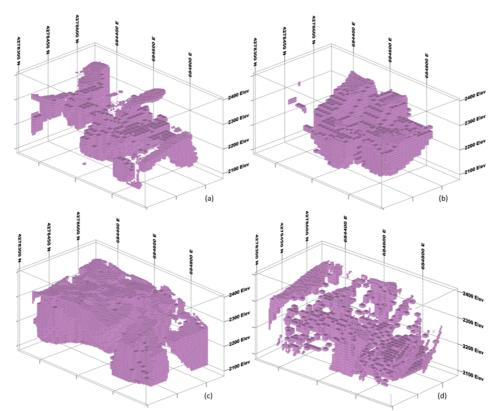
Figure 16. 3D visualization of anomalous zones for (a) electrical resistivity, (b) chargeability, (c) magnetic susceptibility, and (d) Cu grade.
