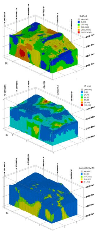
Figure 8. 3D visualization of geophysical models of (a) electrical resistivity, (b) chargeability, and (c) magnetic susceptibility.
