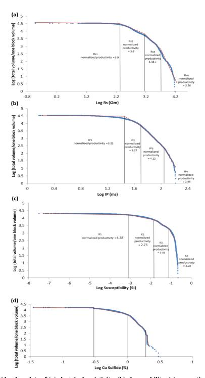
Figure 11. The C-V log-log plots of (a) electrical resistivity, (b) chargeability, (c) magnetic susceptibility, and (d) Cu grade. The normalized productivity values for each zone have been superimposed on the plots.
