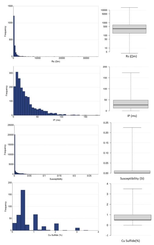
Figure 4. Statistical charts of histogram plot and box-plot for the electrical resistivity (1st row), chargeability (2nd row), magnetic susceptibility (3<sup>rd</sup> row), and Cu concentration (4th row).
