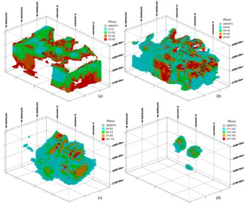
Figure 13. 3D visualization of the multi-fractal models of chargeability, where each model has been re-classified into new populations based on the fractal threshold values (a) first fractal zone; (b) second fractal zone; (c) third fractal zone; and (d) fourth fractal zone.
