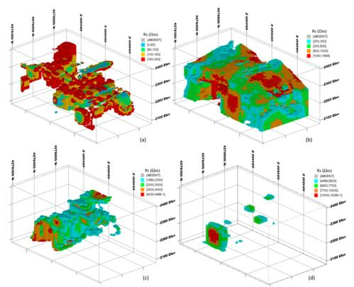
Figure 12. 3D visualization of the multi-fractal models of electrical resistivity, where each model has been reclassified into new populations based on the fractal threshold values (a) first fractal zone; (b) second fractal zone; (c) third fractal zone; and (d) fourth fractal zone.
