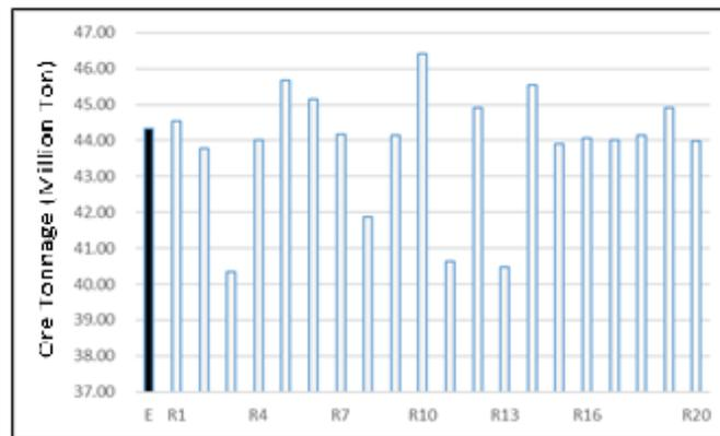
**Figure 3. Total Ore Tonnage in UPL (E: estimate, Ri: Realization i).**
