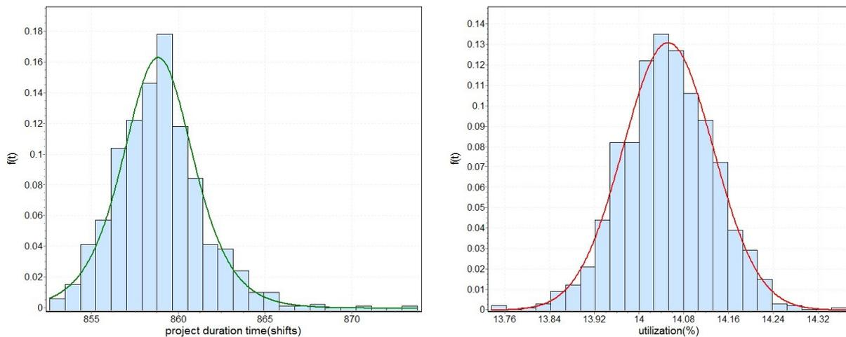
Figure 5. Probability distribution for simulation of project duration and TBM utilization.
