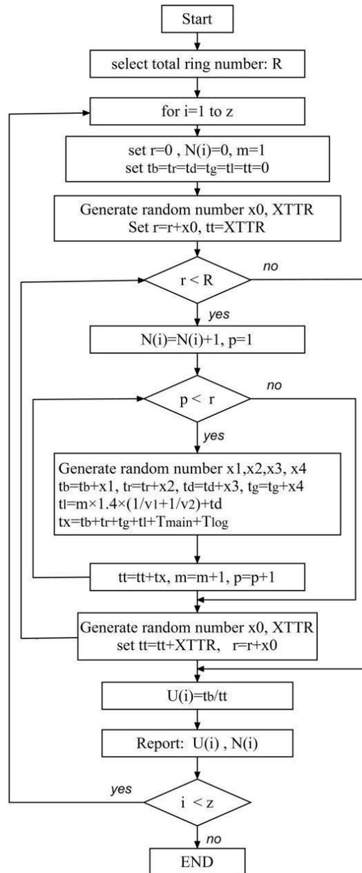
Variables: z: number of simulation, R: total ring number, U(i): utilization factor, N(i): number of stoppage, r: number of ring between stoppage, XTTR: time to repair for cutting tools change, x1, x2, x3, x4
