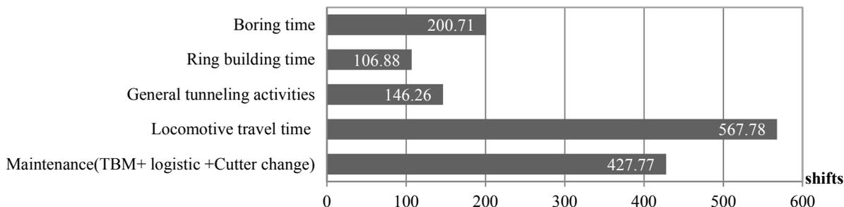
Figure 6. Project duration time details for 5600 meters excavation of tunnel (total time: 1449.4 shifts).
