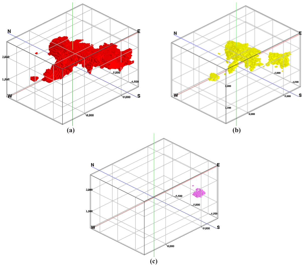
Figure 5. Copper mineralized zones based on S-V modeling: a) major hypogene; b) supergene enrichment; c) skarn.
