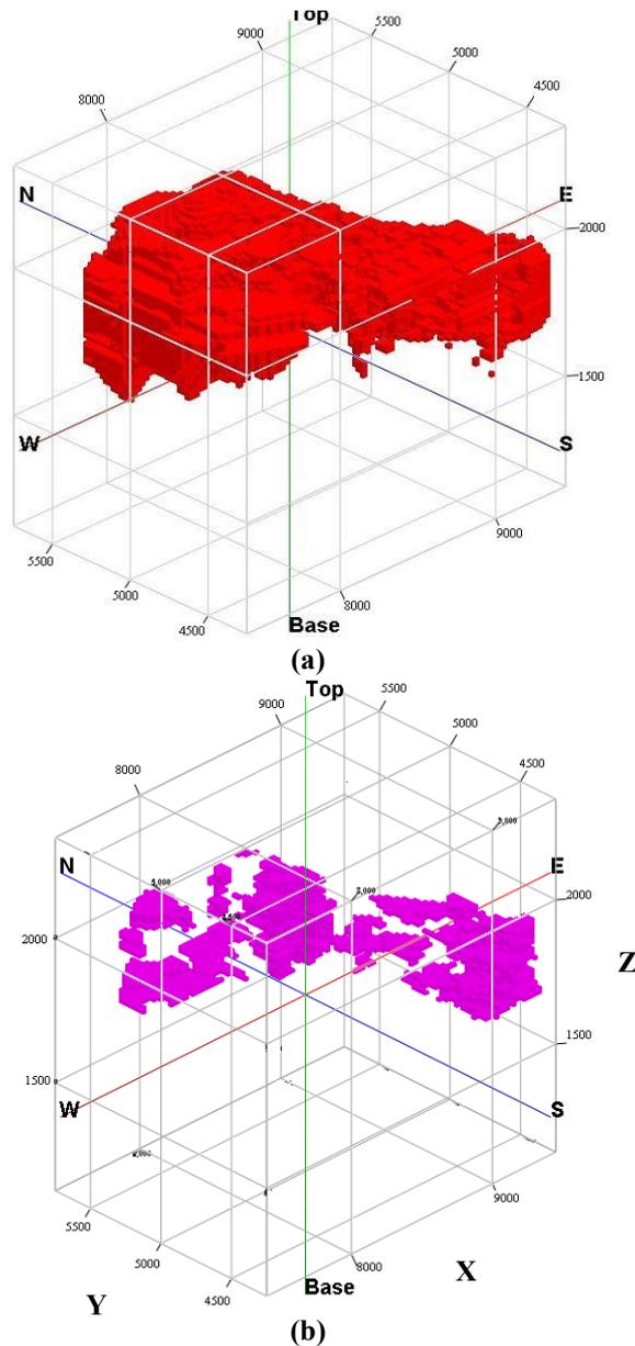
**Figure 3. Porphyry stock (a) and skarn zone (b) 3D models in Sungun deposit based on geological data (coordinate is UTM system).**
