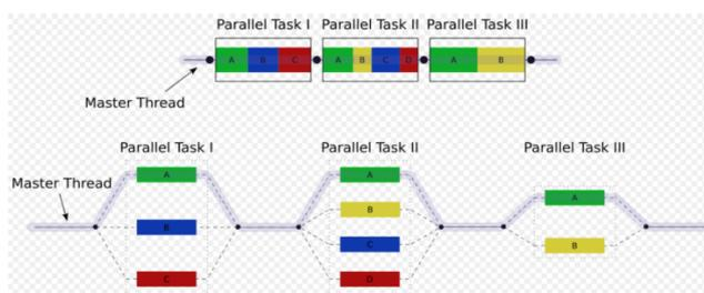
Figure 1. Threads in OpenMp [22].
