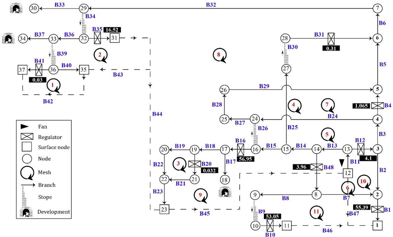
**Figure 3. Locations of fan and regulators in Western-Razmja coal mine.**
