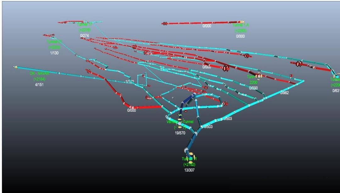
Figure 4. Airflow distribution in Western-Razmja coal mine (VENTSIM 3D).
