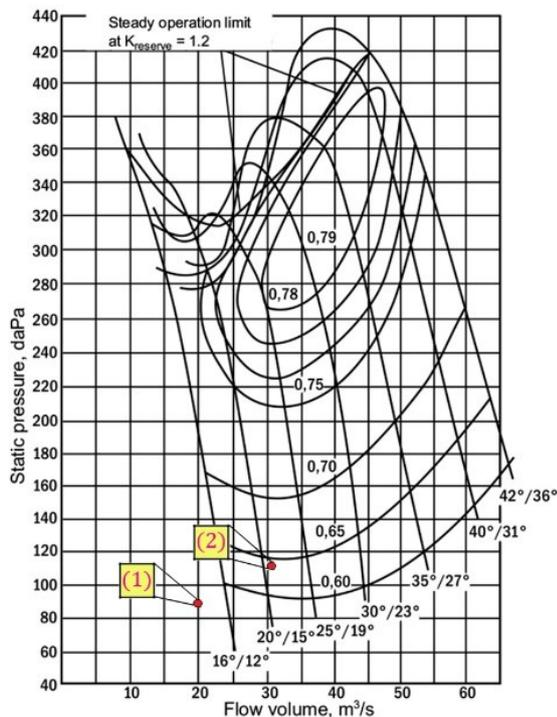
Figure 6. Total efficiency of fan 1: manual method 2: mathematical formulation.
