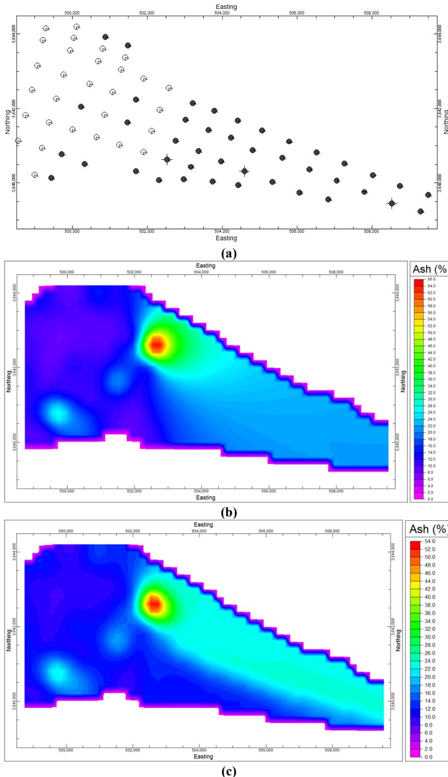
Figure 5. Location of drilled holes (a) and ash distribution maps based on AIDS (a) and OK (b).
