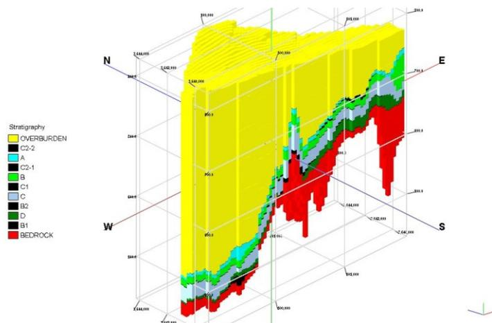
Figure 2. A 3D geological model for the East-Parvadeh deposit with a vertical exaggeration equal to 30 [13].
