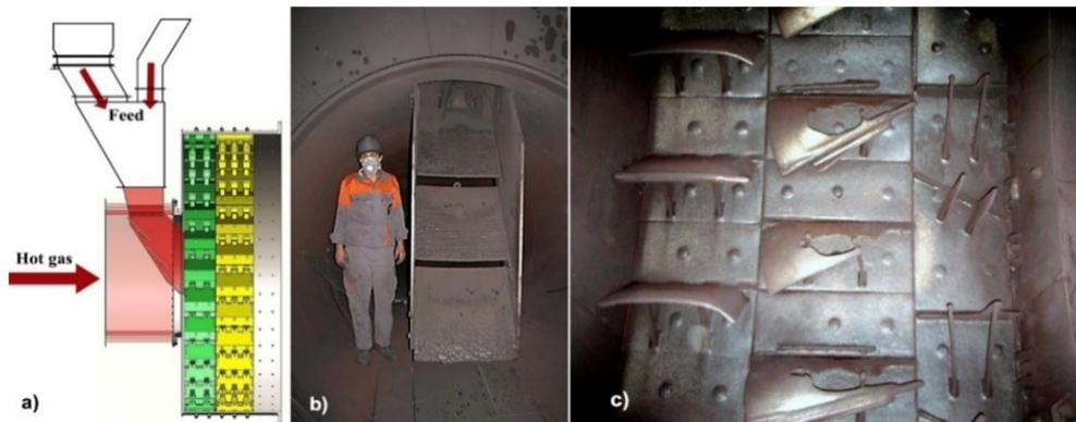
Figure 1. a) Schematic view of dryer and feed chute, b) feed chute, and c) worn dryer flights.
