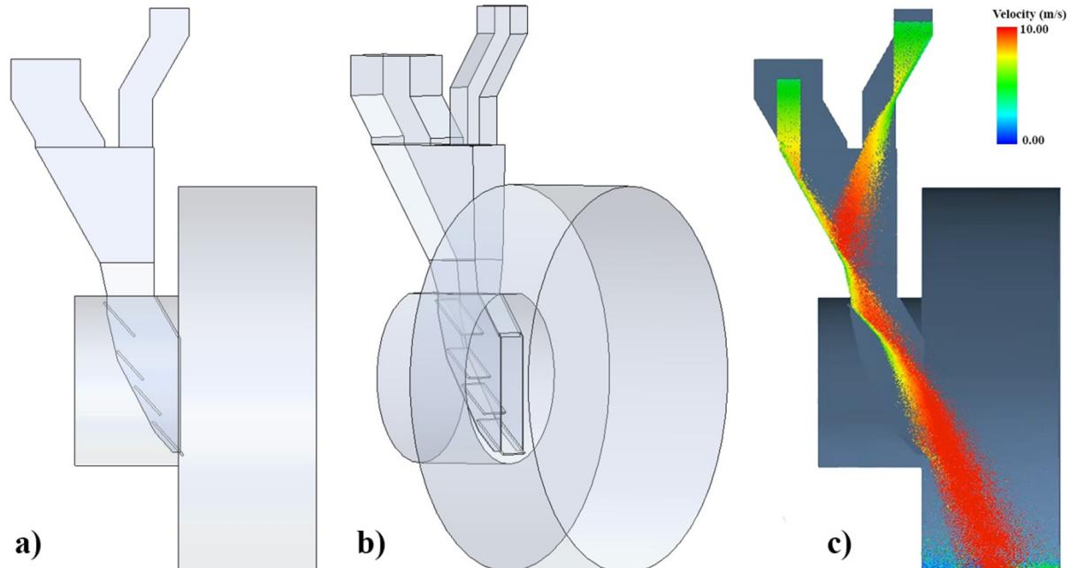
**Figure 4.** The modified feed chute design a) side view, b) perspective view, and c) DEM simulation results.
