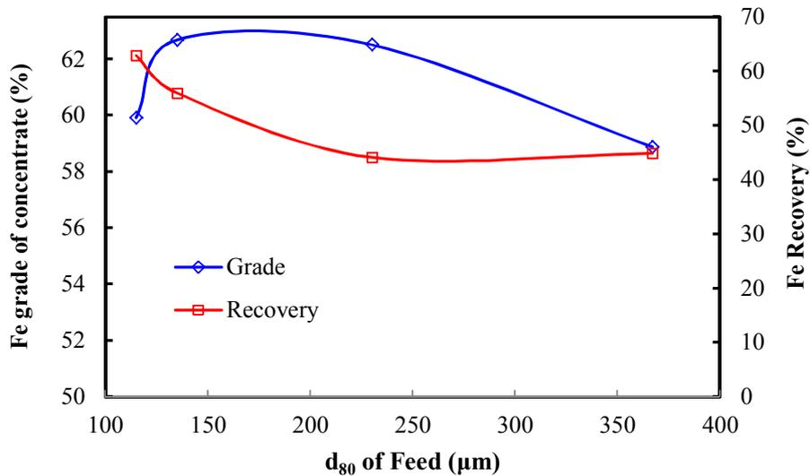
Figure 6. The effect of feed size on the performance of wet low-intensity magnetic separator.
