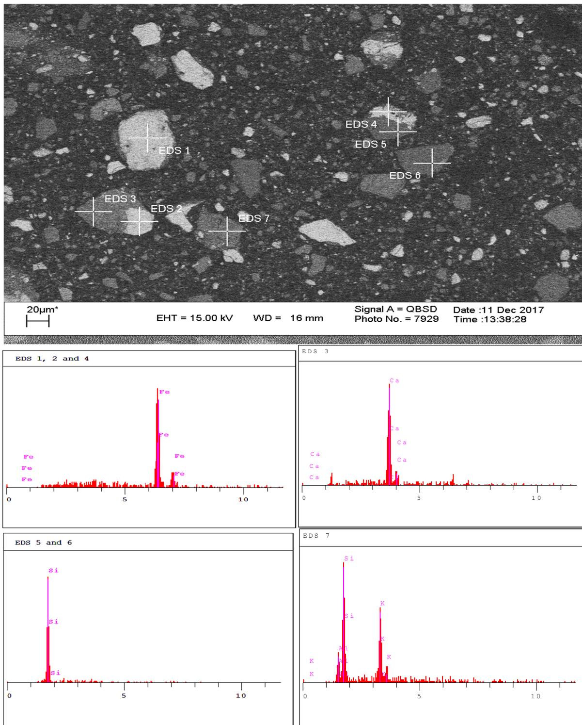
Figure 4. SEM-EDS analysis of the low-grade iron ore sample.
