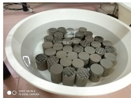
Figure 3. A water bath for saturation of specimens.
