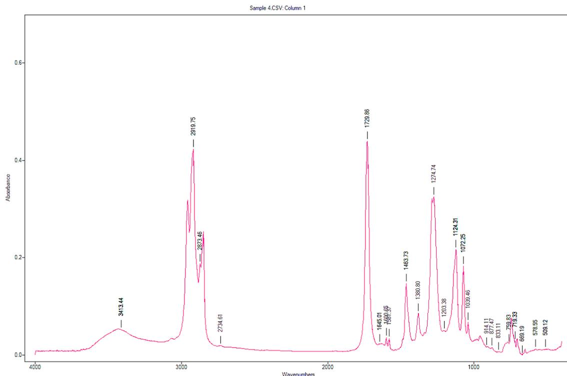
Figure 10. FT-IR spectra of the phase 4 (hexane) extraction.
