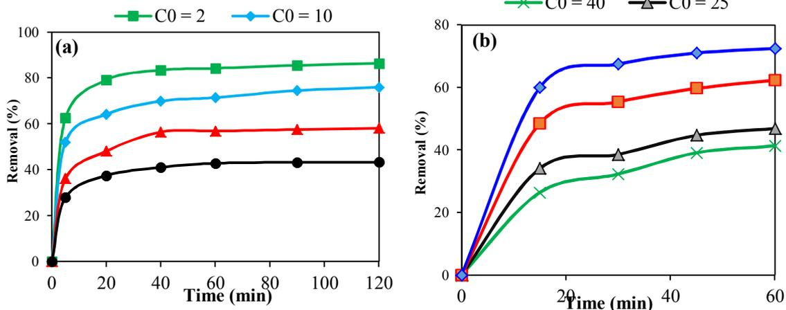
Figure 6. The effect of contaminant initial concentration on the sorption of MB (a) and Ni(II) (b) by ABFDB sorbent.
