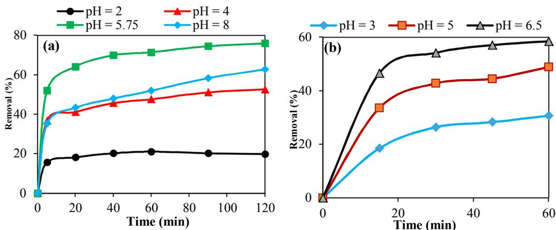
Figure 4. The effect of pH on the adsorption of MB (a) and Ni(II) (b) by *ABFDB* sorbent.
