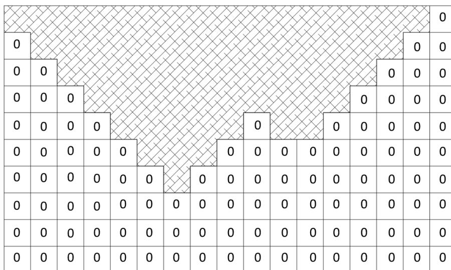
**Figure 3. A cross section of final pit using the traditional objective function**
