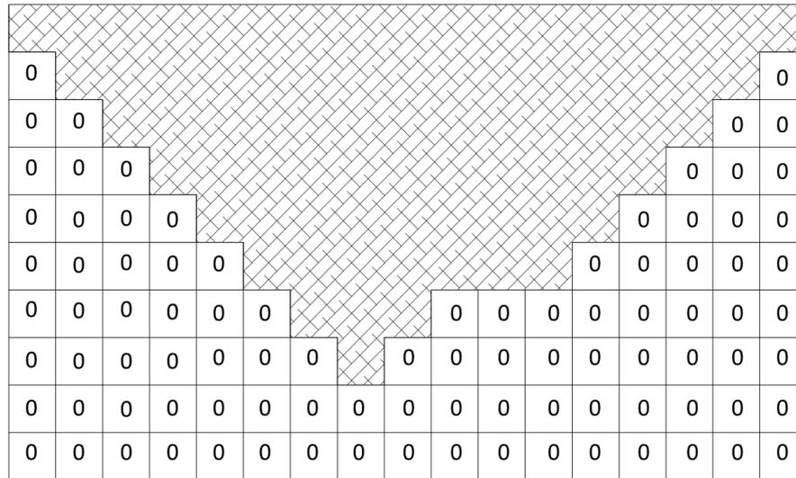
Figure 4. A cross section of final pit using the suggested objective function
