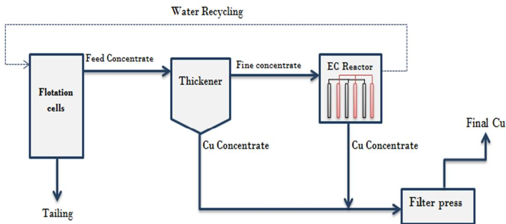
Figure 1. Experimental circuit.
