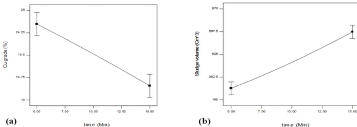
Figure 8. Effect of time a) on Cu grade (%) and b) on sludge volume (electrode type: Fe-Al; current density: 104.10; initial pH: 7), One factor plot
