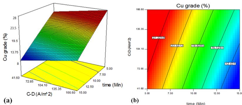
Figure 6. Effect of current density and electrolysis time on Cu grade (%), a) 3D plots and b) 2D contours.
