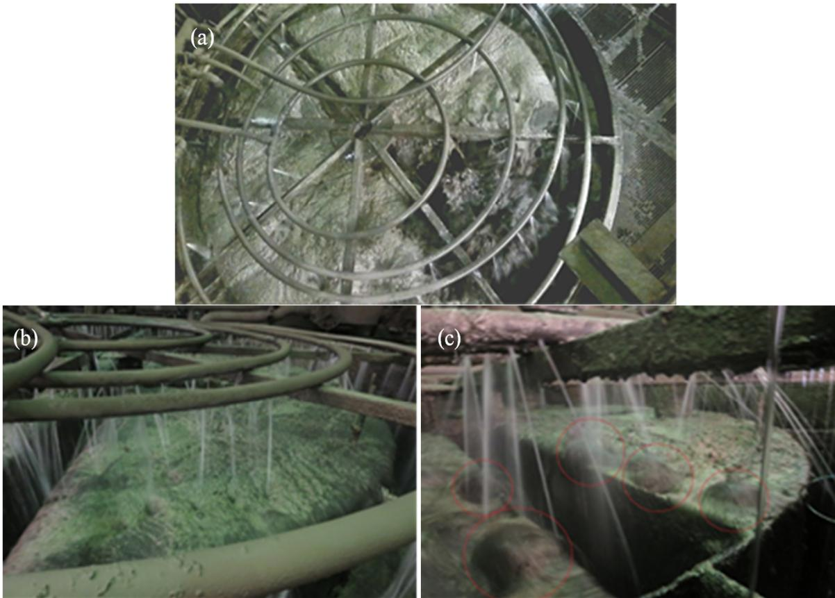
Figure 5. (a and b) burping elliptical column cell. (c) helical column cell No. 2 with uniform air destitution.
