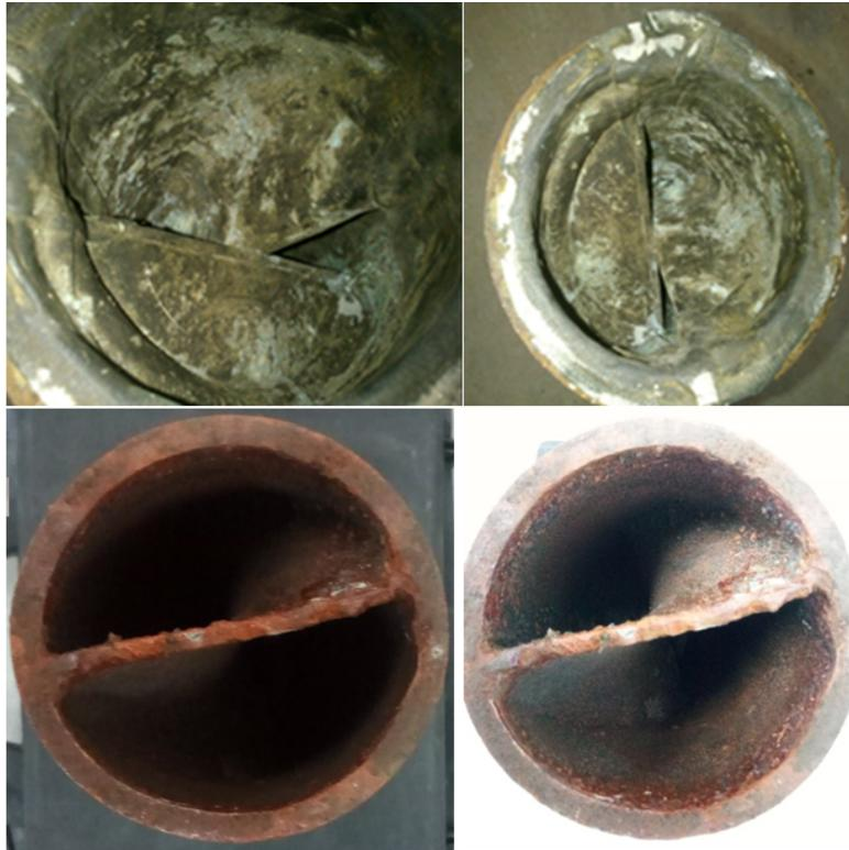
Figure 6. Static mixer of elliptical type (above) after 5 day with choking and helical type (below) after 3 months without choking.
