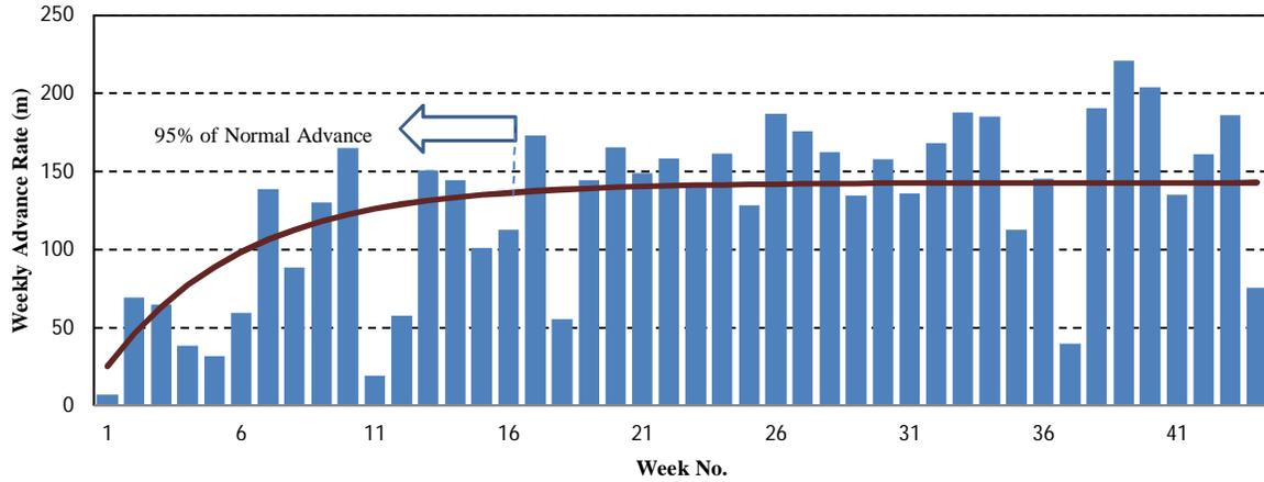
Figure 8. Learning phase overestimation because of TBM advance rate fluctuations of normal weeks (using the Waise and Wachter fitting function).
