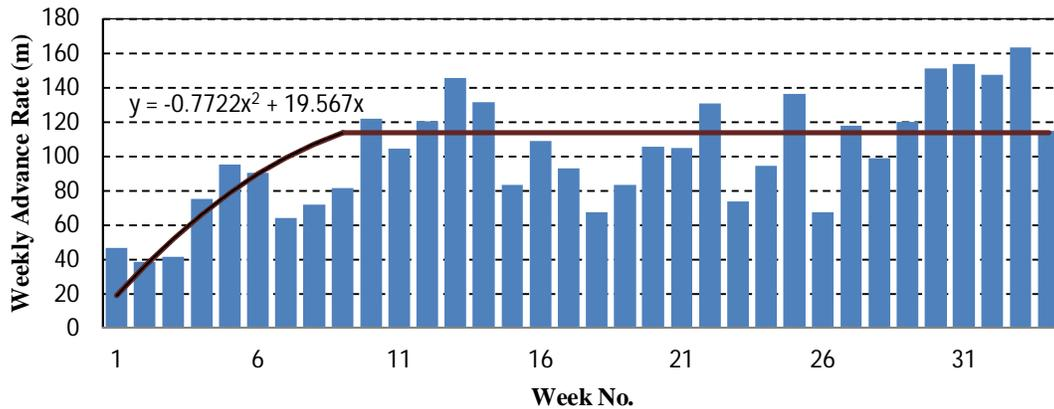
Figure 10. LPP fit function using a polynomial function
