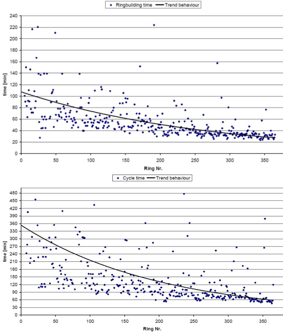
Figure 2. Ring building and cycle times according to the Herrenknecht control system for a tunnel diameter of 5 m excavated by an EPB TBM [23].
