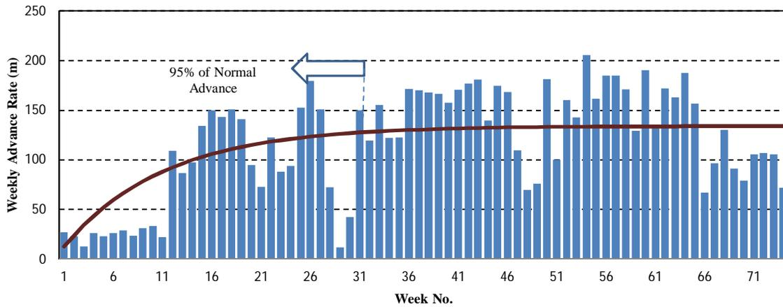
Figure 9. Learning phase overestimation because of unreal shape of learning curve function (using the Waise and Wachter fitting function).
