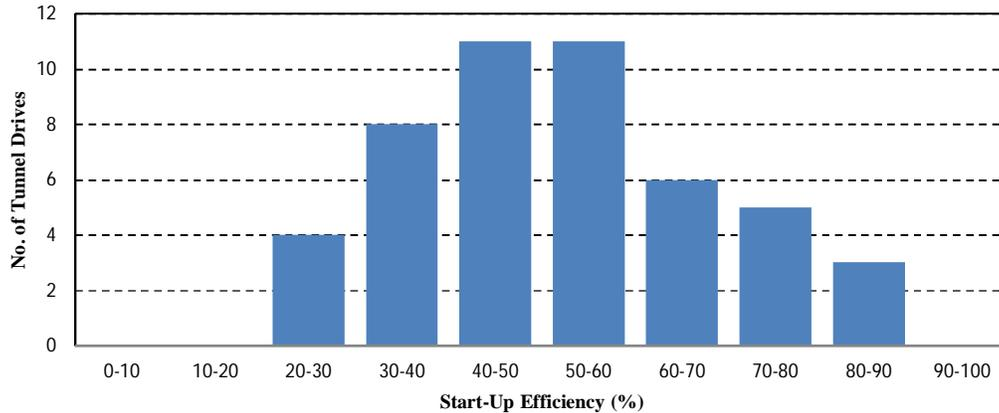
Figure 4. Histogram of start-up efficiency for gripper TBMs according to Laughton [17].
