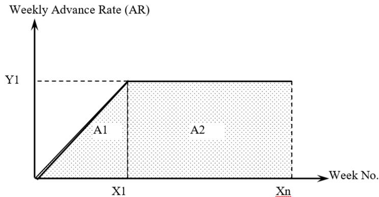
Figure 13. Areas under fitting functions.
