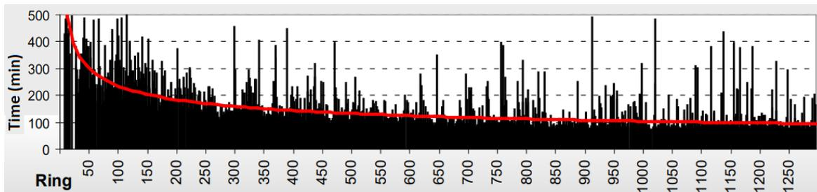
Figure 3. Ring building and cycle times according to Brockway [26] for M-30 road tunnel of 15.2 m diameter, excavated by an EPB TBM.
