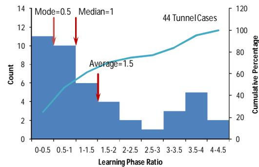
Figure 16. Histogram of distribution of the learning phase ratio for 44 tunnels.
