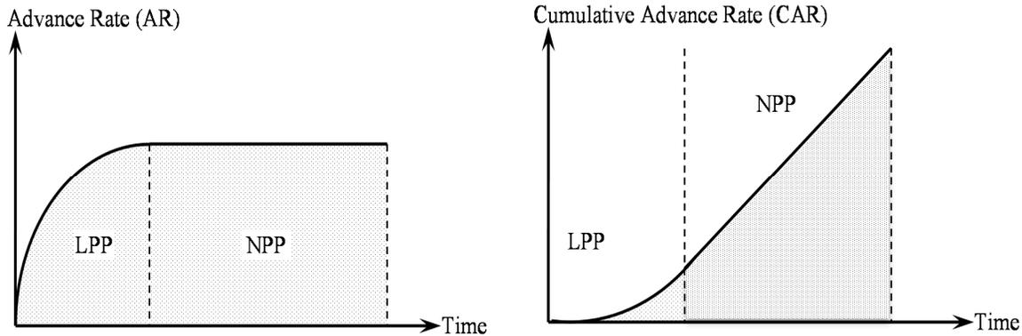
Figure 1. A schematic sketch of LPP and NPP for two common TBM progress diagrams.
