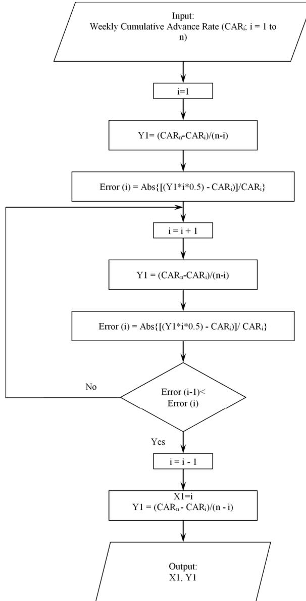
Figure 12. Flowchart of finding the parameters of fitting functions.
