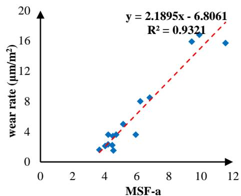
Figure 11. Correlation between  $MSF\_a$  (Equation 9) and wear rate (present study).
