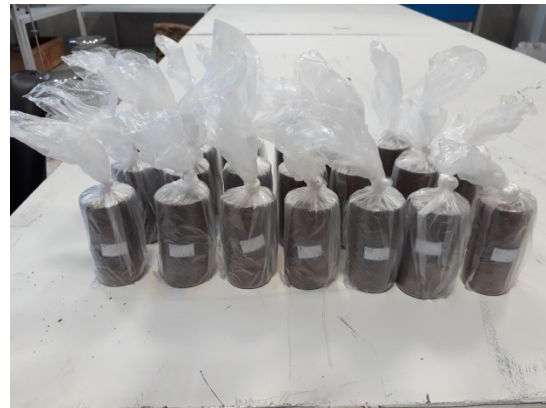
Figure 3. Curing of UCS specimens in nylon bags.
