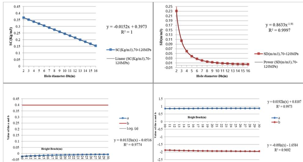
**Figure 3. Relationship of specific charge and specific drilling with hole diameter changes and relations of a and b considering changes of bench height in UCS 70-120 MPa.**
