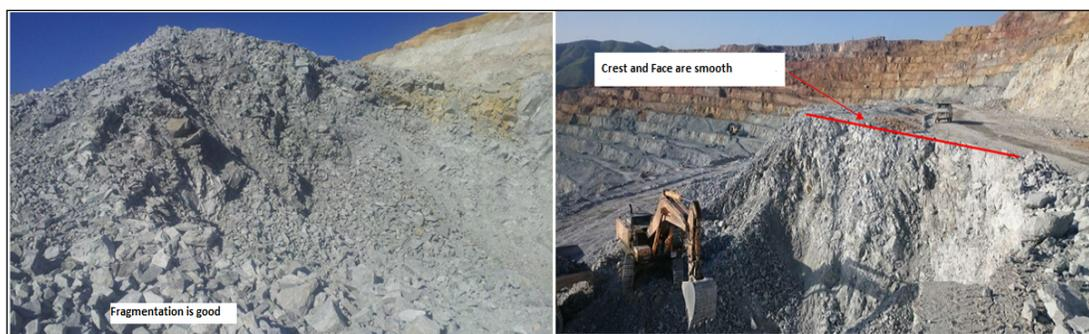
Figure 10. Fragmentation size and the smooth surface after blasting in the level of 2225 m.
