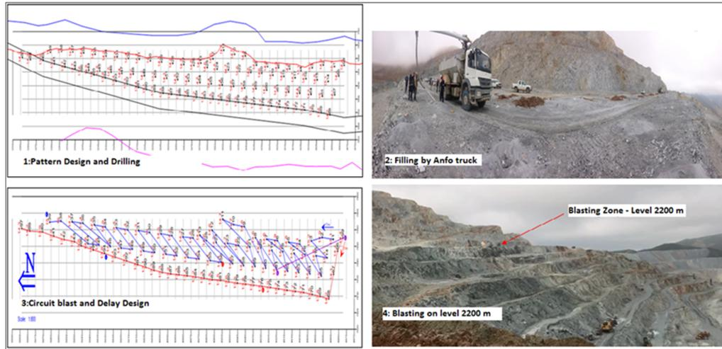
Figure 8. Blasting stages from drilling to the blast in the block in the level of 2200 m.
