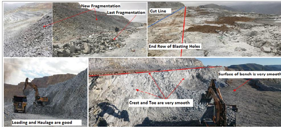
Figure 9. Fragmentation size and the smooth surface after blasting in the level of 2200 m.
