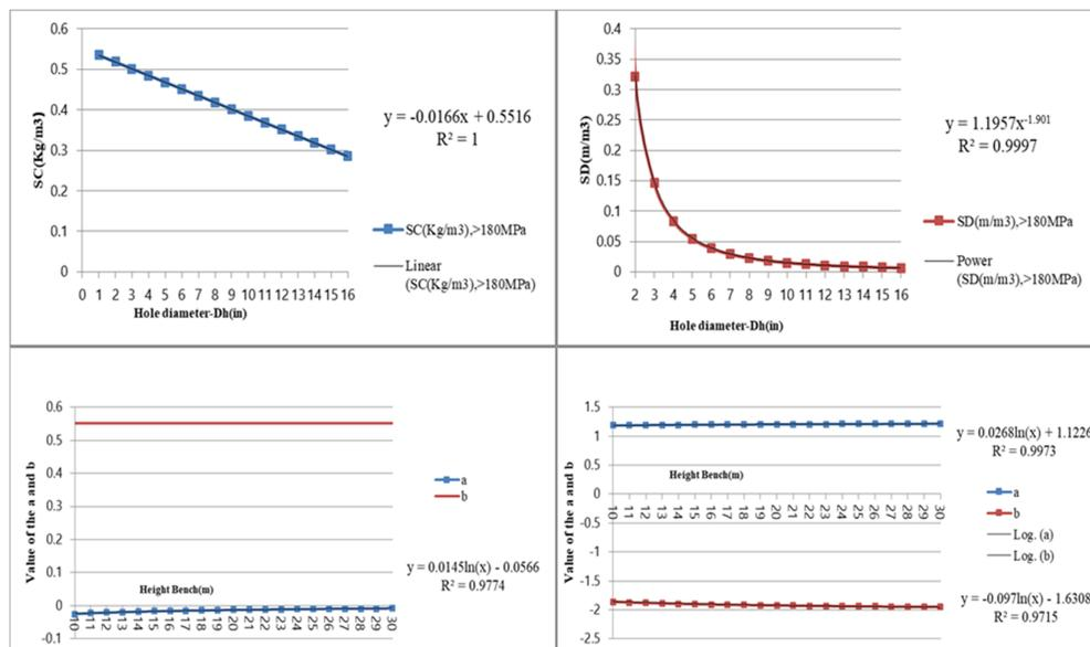
**Figure 5. Relationship of specific charge and specific drilling with hole diameter changes and relations of a and b considering changes of bench height in UCS 180-250 MPa.**
