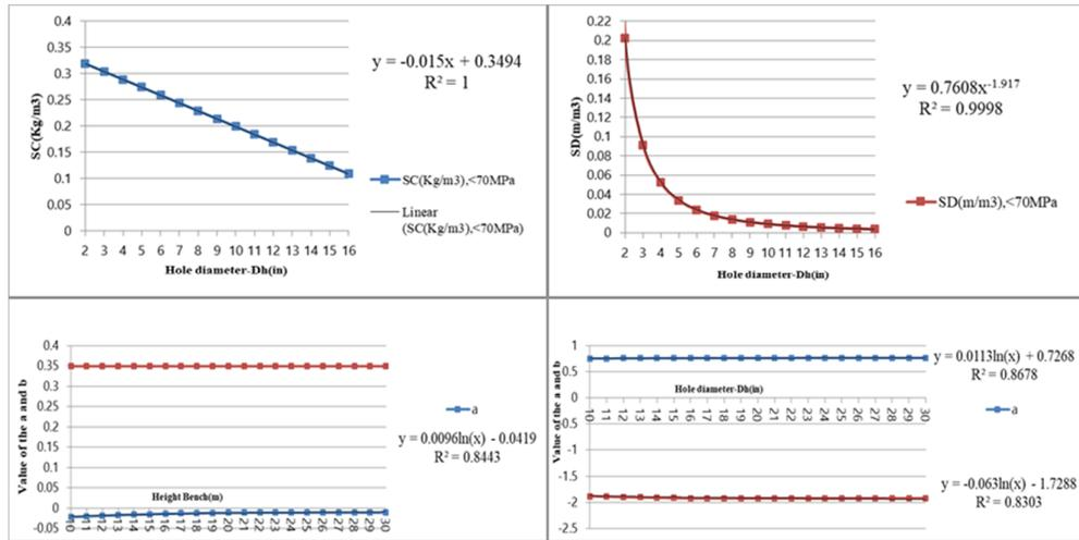
**Figure 2. Relationship of specific charge and specific drilling with hole diameter changes and relations of a and b considering changes of bench height in UCS 10-70 MPa.**
