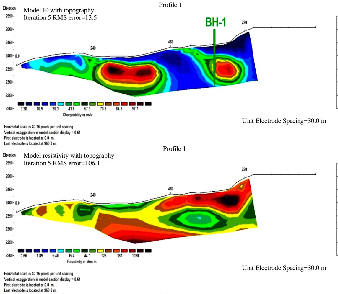
**Figure 11. Inverted values of geophysical data using the Res2DInv software for profile 1.**
