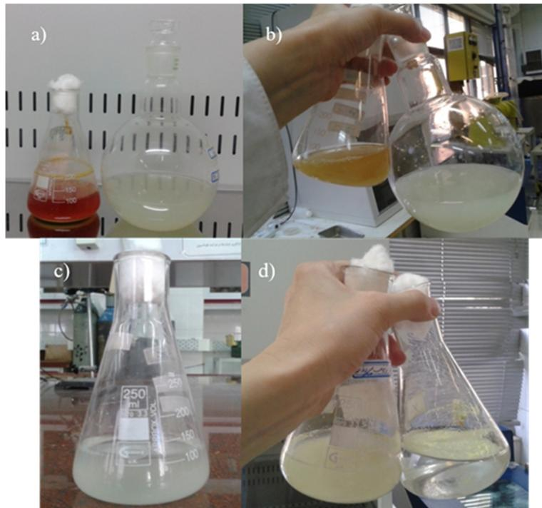
**Figure7.** a) Comparison between primary 9KFe medium and culture medium by incomplete growth after 30 days; b) Comparison between primary 9KFe medium and culture medium by complete proliferation after 30 days; c) Comparison between primary 9KS medium and culture medium by incomplete growth after 30 days; d) Comparison between primary 9KS medium and culture medium by complete proliferation after 30 days.
