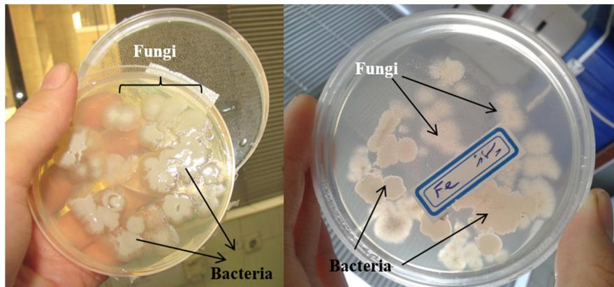
Figure10. Cultivation of bacteria from the 9KFe medium in the solid nutrient agar.
