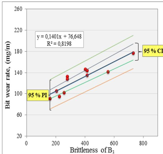
Figure 4. Correlation between the bit wear rate and the brittleness of the B<sub>3</sub> tests within a 95% CI and 95% PIs.
