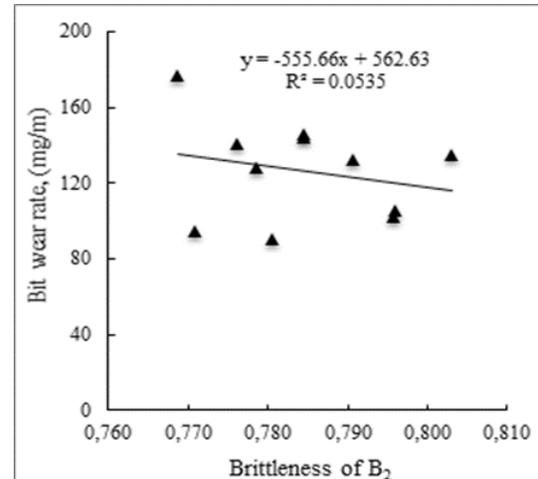
Figure 5. Correlation between the bit wear rate and the brittleness of B<sub>1</sub> and B<sub>2</sub>.
