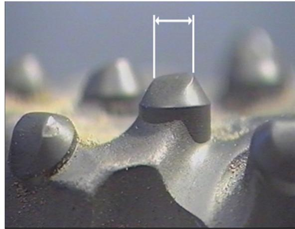
Figure 7. Button tip wear in button bits.
