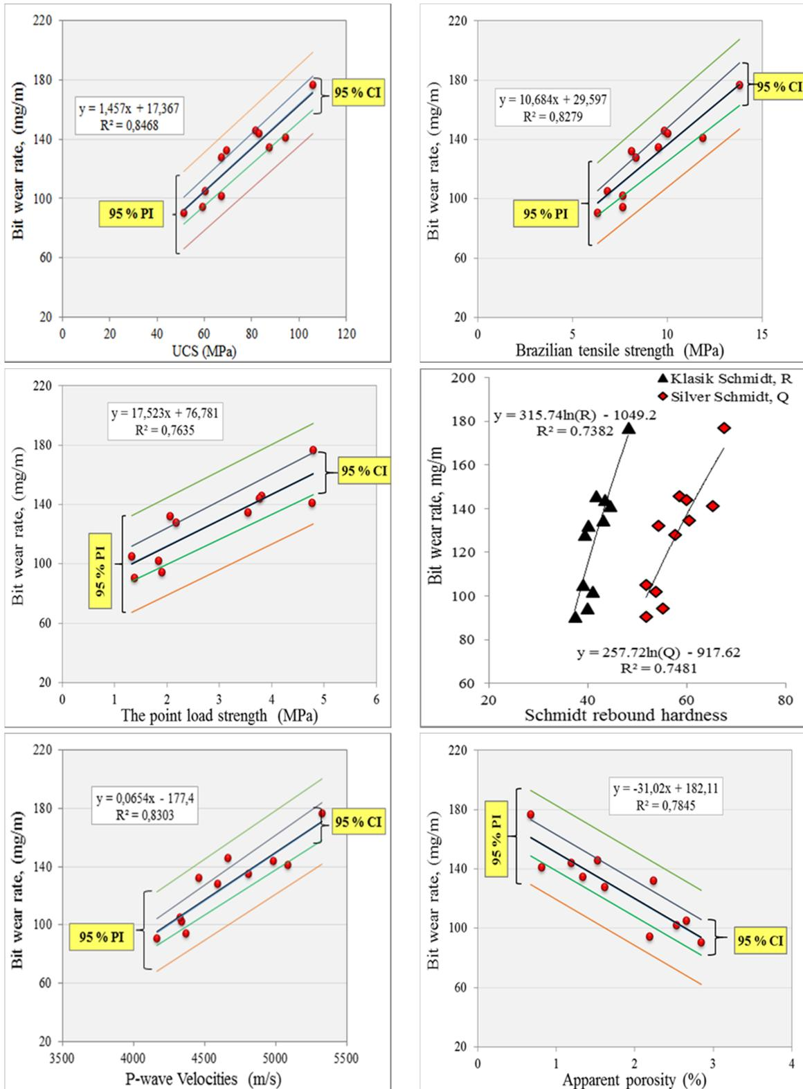
Figure 1. Bit wear rate correlation with the physical-mechanical property tests within a 95% confidence interval (CI) and 95% prediction intervals (PIs).
