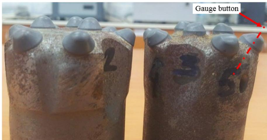
Figure 6. Gauge buttons of drill bits.
