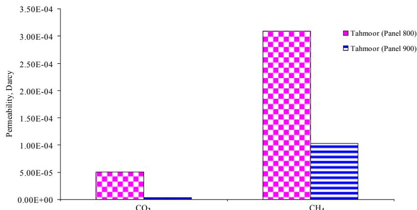
Figure 9. The permeability test results for 800 and 900 panels coal samples (Tahmoor Colliery) under 100 kg axial load and 0.5 MPa gas pressure.
