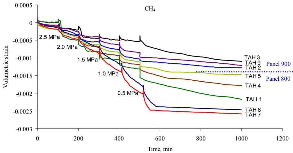
Figure 4. Volumetric strain for CH<sub>4</sub> and pressure reductions at increments of 0.5 MPa
