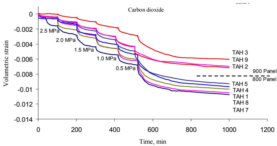
Figure 3. Volumetric strain for CO<sub>2</sub> and pressure reductions at increments of 0.5 MPa
