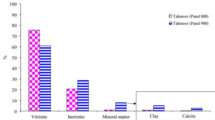
Figure 7. The petrographical test results for Tahmoor Colliery coal samples
